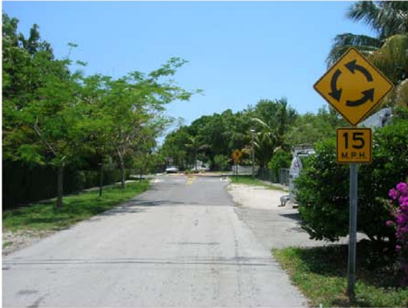
Recently built traffic circles force neighborhood traffic to slow down.
