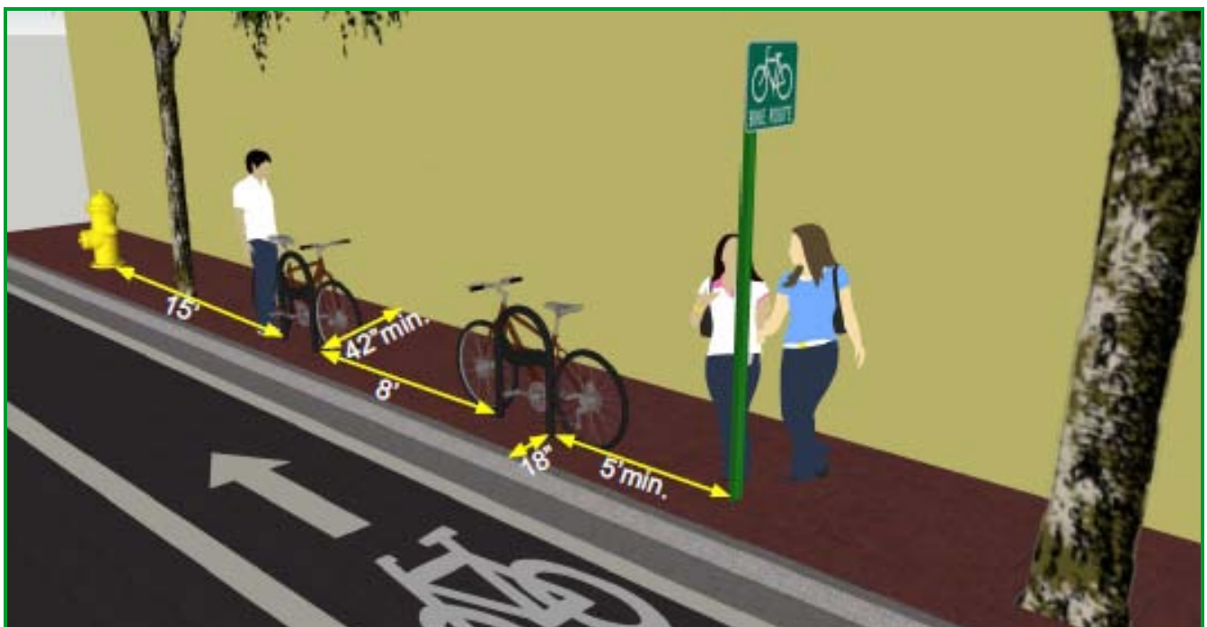
Figure 7- 14: Narrow Sidewalk Dimensions for Specific Bicycle Parking Guidelines
