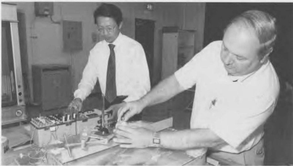
Milton Torres (right) and Kuang-Hsi Wu (left) test the flexibility and strength of a sample piece of aircraft skin treated with the polymer.
