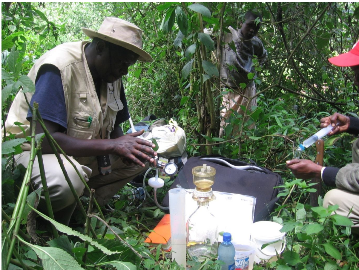
Figure 8: Filtration on site for suspended solids (left) and DOC right
