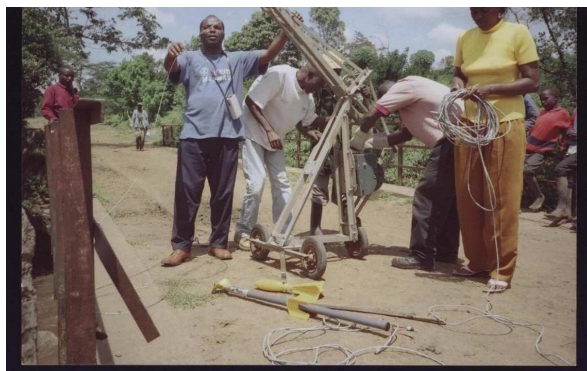
Figure 4. 2. Preparing a bridge crane to lower USDH-59 Sediment Sampler after current meter (in the foreground) has been used in gauging.
