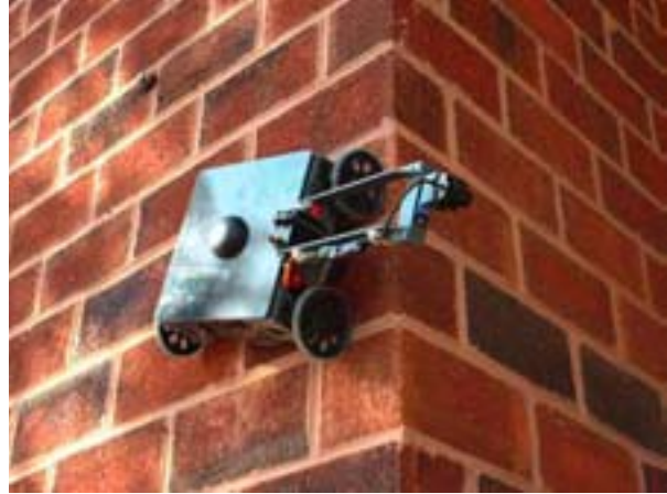
Clarifying Climber III Remote-controlled climbing robot Robot-mounted roaming cameras can feed video data into LCD screens or projections against floor and wall surfaces throughout the airport terminals.
