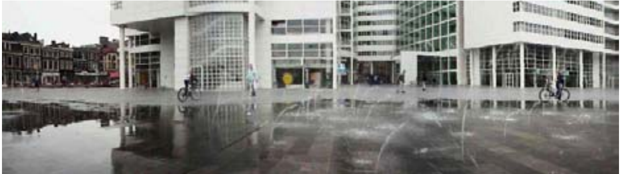
Peter Struycken Spuiplein, Den Haag, Netherlands Constantly-changing, regular grid of 14 x 14 water nozzles, 196 water pumps, controlled by 8-bit microprocessors
