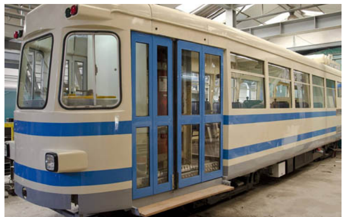
FIGURE 4.31: SPANISH NATIONAL RAIL OPERATOR FEVE'S PROTOTYPE HYDROGEN FUEL CELL TRAM
