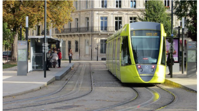
FIGURE 4.29: ALSTOM APS GROUND-LEVEL SYSTEM IN REIMS, FRANCE
