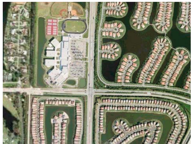
Sprawl: Streets do not often connect, and all trips are forced on a collector road.
