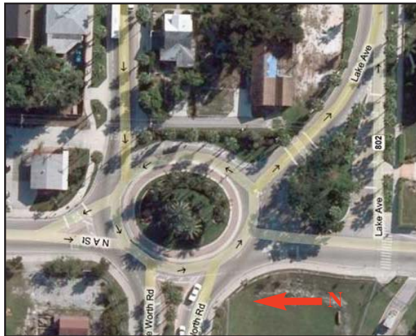
Deflection or forcing the car to turn around the roundabout is the key to speed control. As apparent in this diagram, the approaches from the north and east have little or no deflection.
