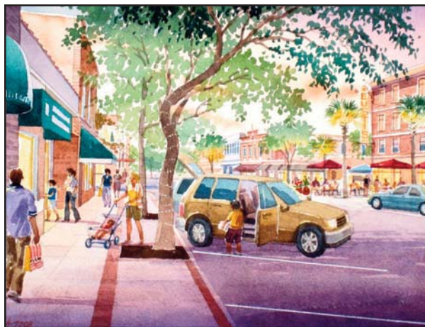
Back-in angle parking is safer than front-in angle parking for loading and unloading and easier to maneuver.
