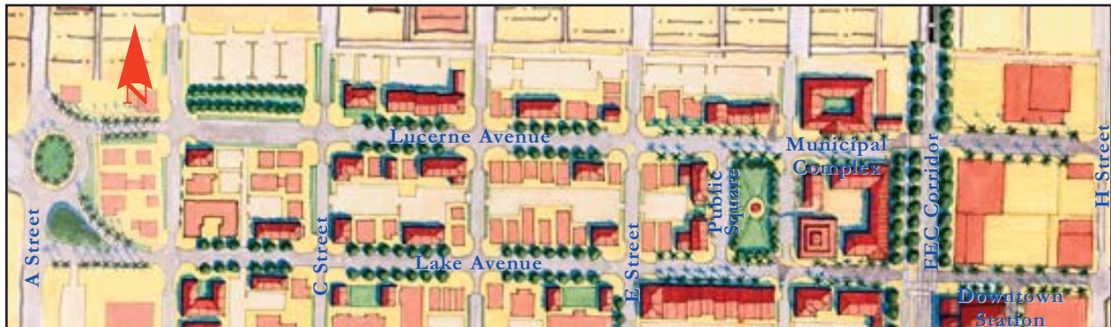
Above is a detail of the Citizens' Master Plan for the Lake Avenue West district. Note the new public street and square immediately west of the proposed city hall and municipal complex. The rendered roofs represent new construction while the non-rendered roofs are existing buildings to remain.
