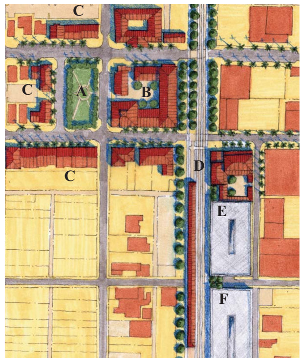
This image is a detail of the city hall and new public square plan as it relates to the proposed “Town Center” station and the future parking garages east of the FEC tracks: A). New public square; B). New city hall; C). New redevelopment around public square; D). “Town Center” station; E). Phase I garage; F). Phase II garage for new city hall and municipal complex.
