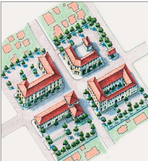
Buildings shielding parking provides convenient access by car and helps the street by creating a street facade for pedestrians
