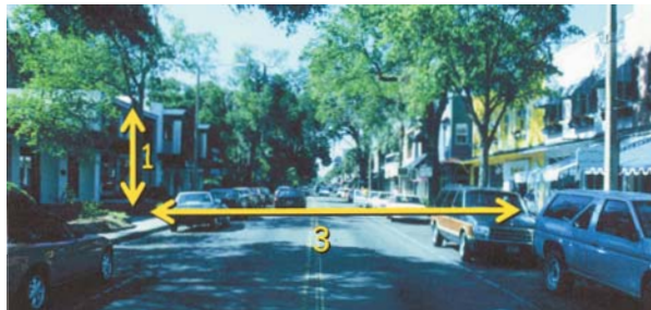
According to Architectural Graphic Standards , a ratio of one-to-three is the minimum if a sense of spatial enclosure is to result. The smaller the ratio is, the better.
