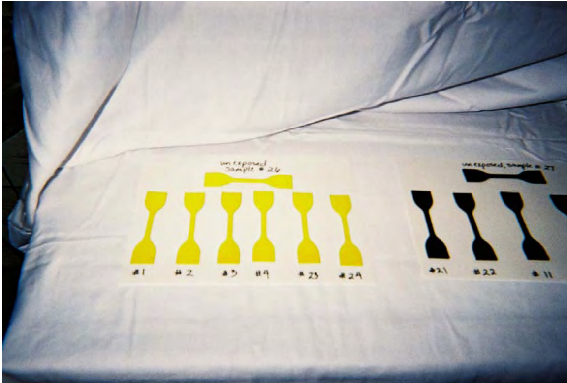
Figure 5-11. Post testing for material #1. An unexposed sample is at the top for comparison.
