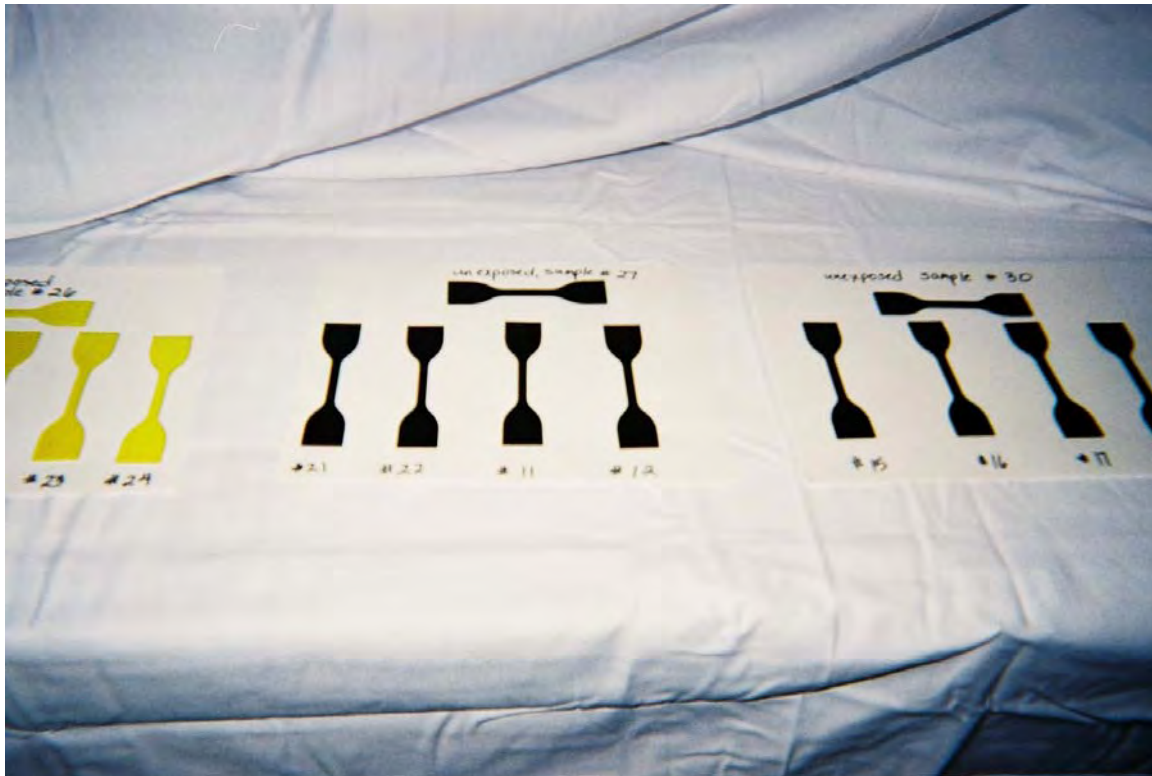
Figure 5-12. Post -testing for material #2. An unexposed sample is at the top for comparison.
