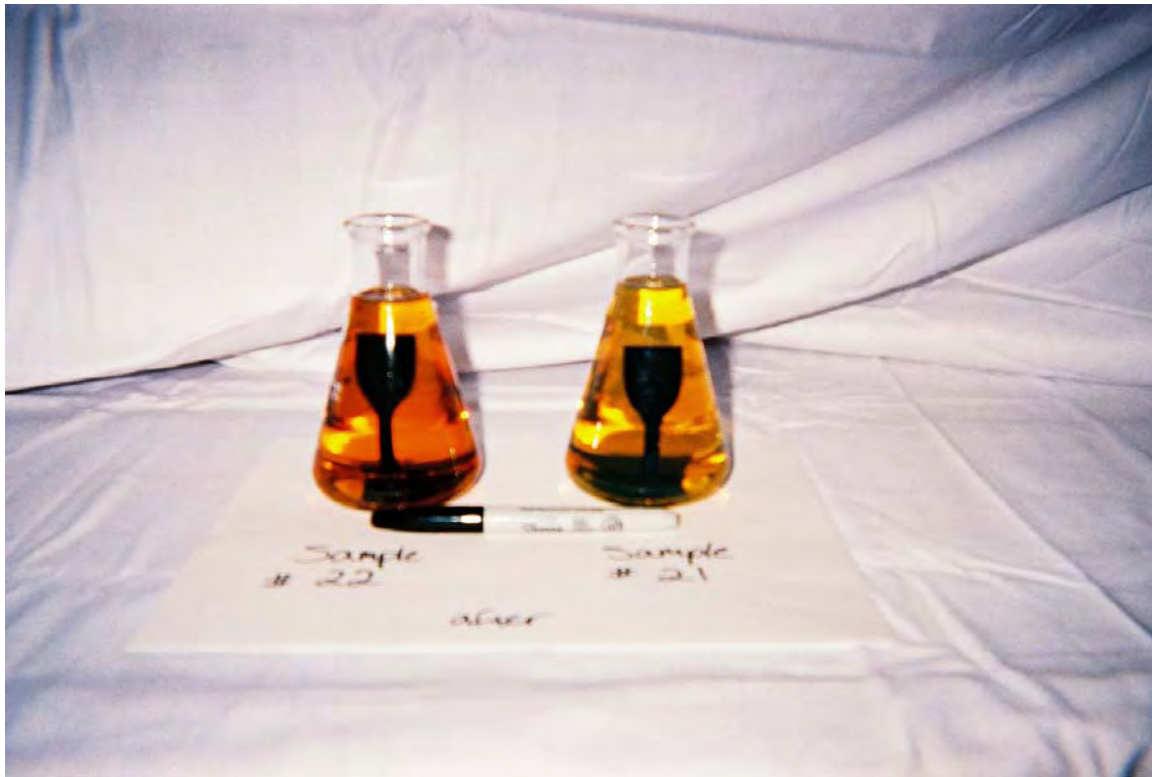
Figure 5-10. Material #2 post-testing. Low-sulfur diesel on the right, blend with biodiesel on the left.
