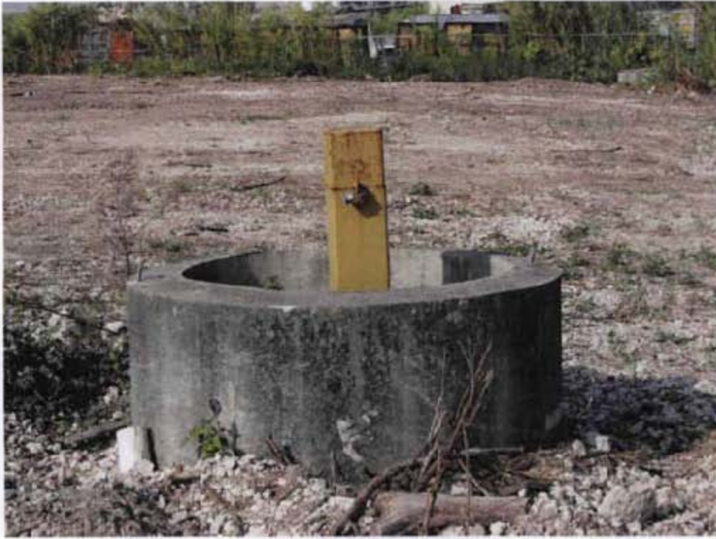
Monitoring well on top of the monolith in the Curtis parcel.
