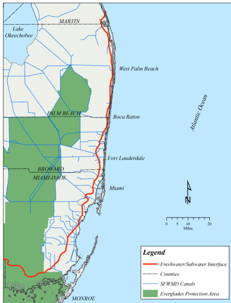
Figure 5. Estimated freshwater/saltwater interface in the lower east coast for the years 1995 through 2000 based on measurements from 100 mg/L chloride to 250 mg/L chloride and above. (Map produced by the SFWMD.)
