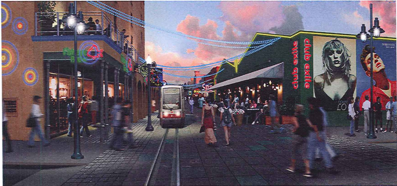
This illustration shows how a narrow gauge rail vehicle can be small enough to fit within narrow right-of-way.
