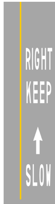
Pavement markings, like these shown above, will be used as traffic calming devices in constrained or limited-visibility areas, such as locations where the M-Path meanders through the Metrorail support columns.
