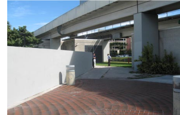
Opaque walls, like the one shown above, limit the ability of trail users to see what is around them. Conditions like this may cause M-Path users to feel unsafe and may encourage criminal activity.
