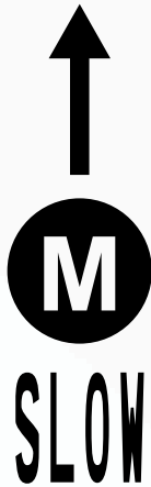
Pavement marking for Metrorail station plaza approaches.
