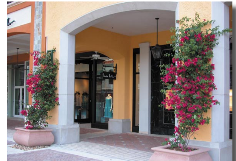
Arcades should include ample lighting and visibility to the store fronts. Arcades should be wide enough to allow for continuous pedestrian movement as well as provide for seating and displays.
