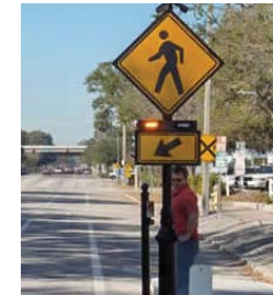
Push button activated stutter signal (flashing beacon)
