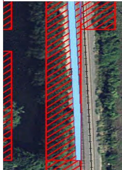
Figure 14: This portion of railroad may only be inundated as a result of the adjacent water body.
