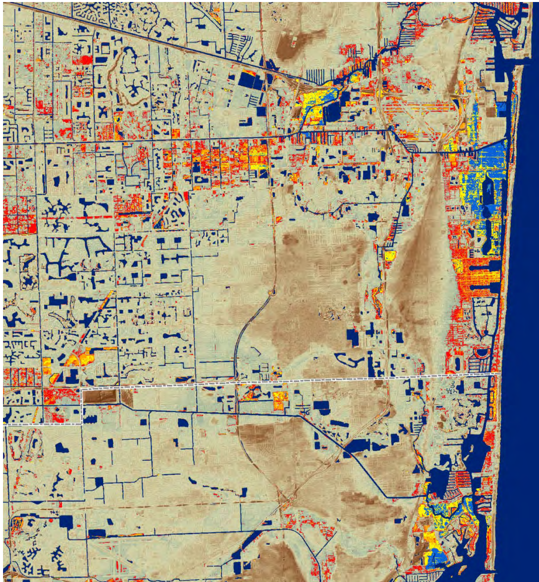
Figure 15 - SLR Vulnerability at 1 to 3-ft above MHHW (Assuming No Elevation Errors)
