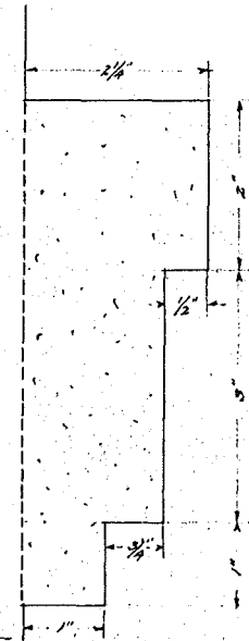
STUCCO MOLDING AROUND FRONT DOOR. FULL SIZE.
