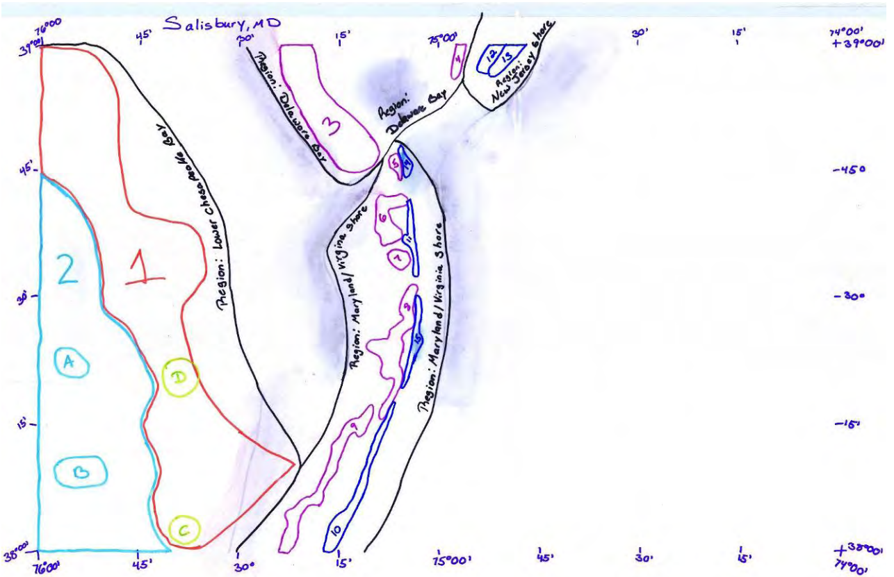
Figure 2.2.1. Polygons Created by Wetland Accretion Panel Assessment: Salisbury Quadrangle. The wetland accretion panel drew polygons on 1:250,000 USGS quads. Panel staff then traced the polygons onto Mylar. The black lines define subregions; the other colored lines define polygons representing wetlands of a given geomorphic setting.
