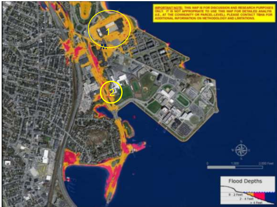
Figure 17. Projected surface flooding from a 5-ft storm surge (MHHW+5/9.8 ft NAVD). Vulnerable areas at UMass Boston are circled in yellow and include the Bayside Expo property (1) and Morrissey Blvd (2).
