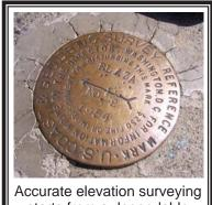
Accurate elevation surveying starts from a dependable elevation reference mark.
