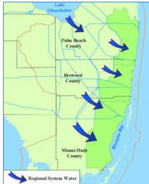
Figure 19 - Billions of gallons of water flow daily through the surficial aquifers from the Everglades to the Atlantic Ocean. (Graphic: SFWMD)
