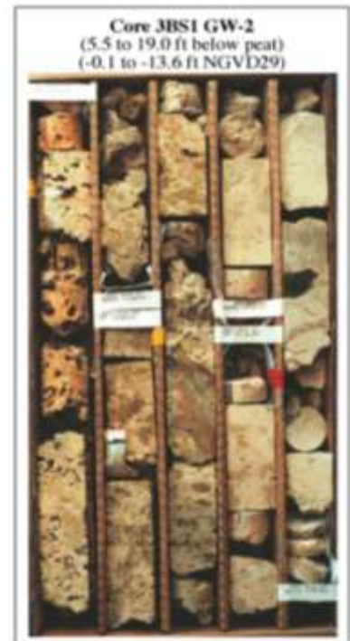
Figure 12 -Biscayne Aquifer is a karst formation with high porosity and variability. (D. McNeill, U. Miami)
