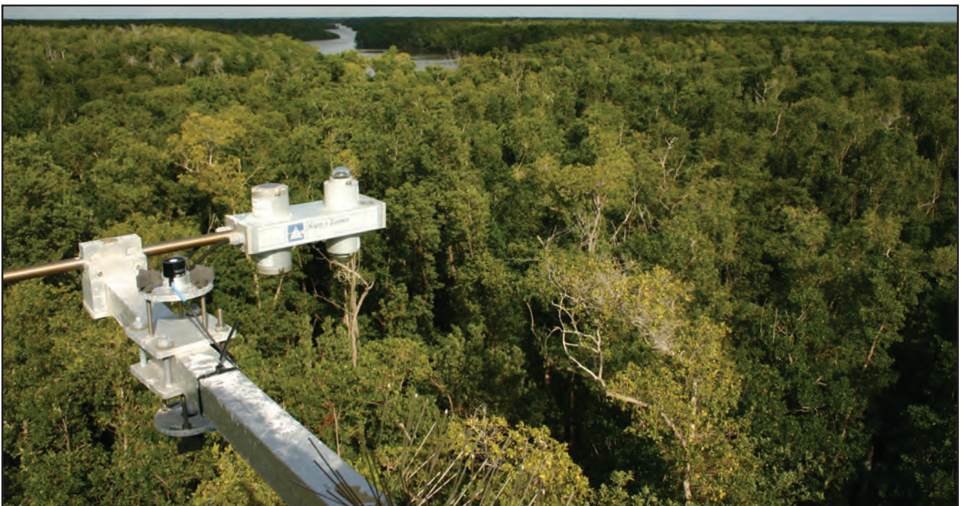
Meteorological instrumentation at the CO 2 flux monitoring station in Shark River Slough. Photo by Jordan Barr, ENP.
