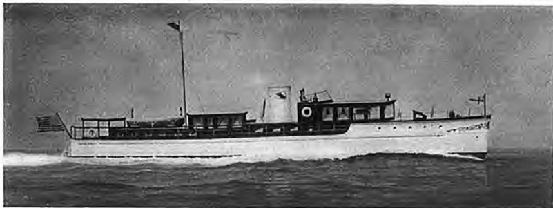
The much to be desired, but previously unobtainable combination of Commuting Speed—Diesel Safety—and Diesel Economy of Operation is today made possible for the first time in history by the use of Treiber Diesel Engines. The beautiful yacht pictured above—85 feet O. A. length by 14 feet beam—is being all Treiber Diesel equipped with Twin 300 H. P., V-type, 12-cylinder Treiber Diesel Propelling Engines and a 7½ K. W. Treiber Diesel Electric Generating Set. Speed 24 miles per hour.
