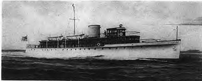
Two V-type, 12 cylinder 16" x 16" Treiber Diesel Engines, each of 2500-3000 H. P. are on order for installation in the yacht illustrated above. It is calculated from model experiments conducted in the U. S. Government testing tank in Washington, D. C. that her Treiber engines will drive her 40 miles per hour, making her by far the fastest Diesel powered vessel ever built. One engine is already completed, has undergone satisfactory shop tests and been accepted by the Owner. The other is in process of construction as this bulletin goes to press.
