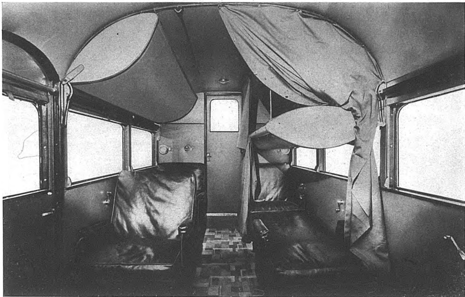
AN INSTALLATION OF SPECIAL EQUIPMENT IN A MODEL 61-C, SHOWING ARRANGEMENT FOR DAY AND NIGHT USE, WITH REMOVABLE PULLMAN TYPE CURTAINS.
