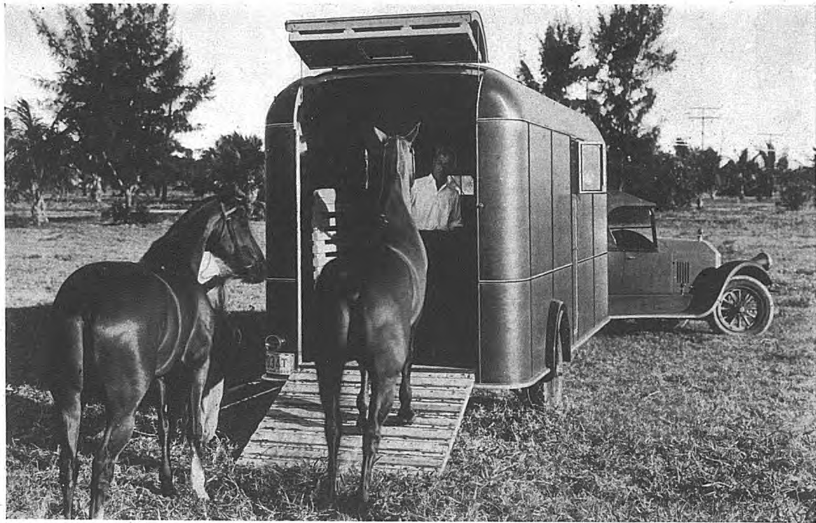
LOADING A MODEL 61-H (NOTE LOW FLOOR).
