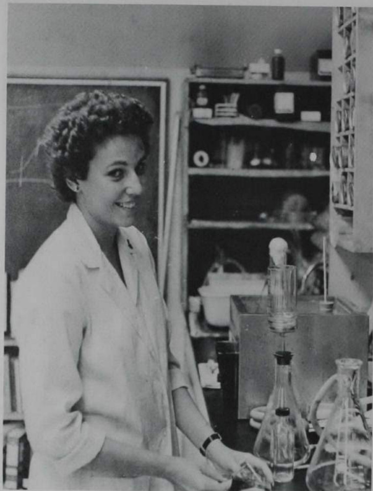
Marister Ruiz is analyzing a sample by passing it through a millipore filter.
