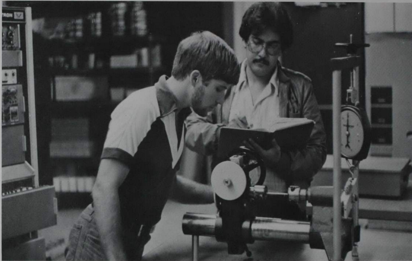
Armando Cruz and Farhad Koucherkpour use the torsion testing machine on steel in their work in the lab.
