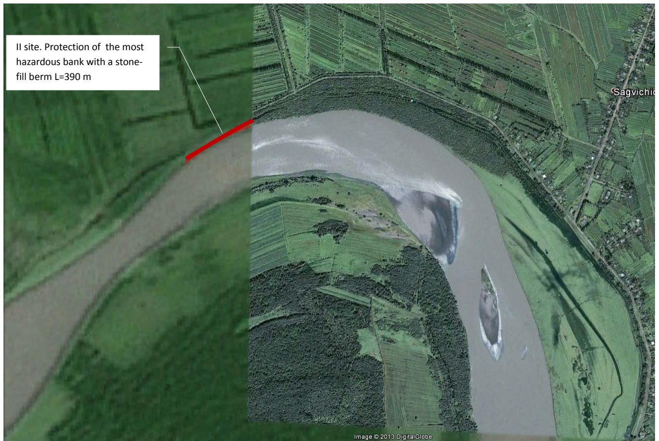
Pic. 8. Village Sagvichio. Suggested bank protection measure at the eroded right bank of the Rioni River
