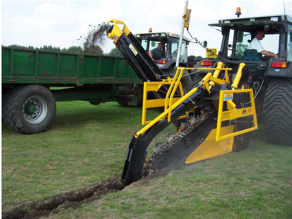
Pic. 6. Example of a special ditching machine
