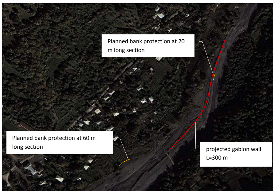
Pic. 17. Village Likhetai. Planned bank protection activities on the Likhunistskali River
