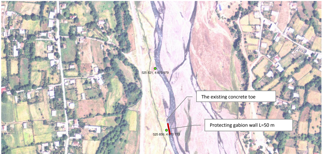
Pic. 21. The scheme of protection of the water distribution well on the right bank of the river in the village Birkiani
