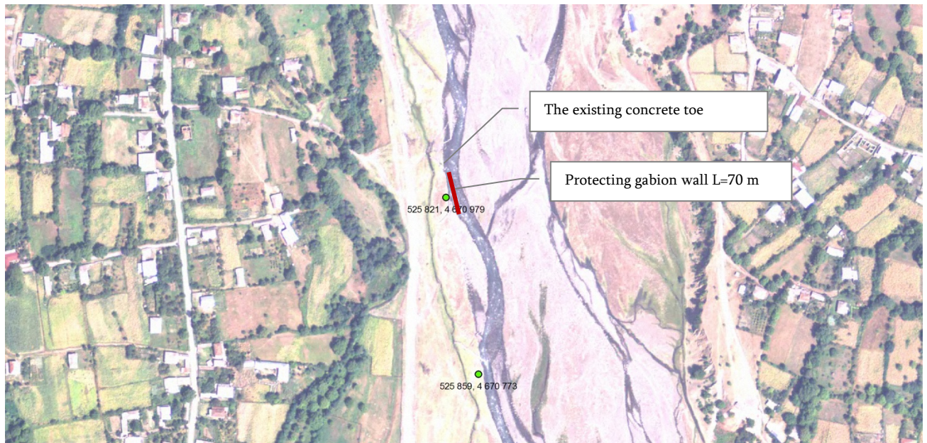
Pic. 20. The scheme of protection of the water distribution well on the right bank of the river in the village Birkiani
