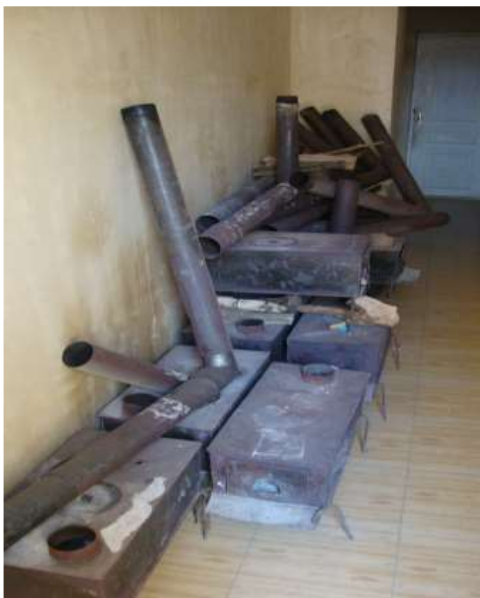
Figure 4.2 Private school in the city of Dedoplistskaro. These are typical inefficient traditional wood stoves invariably used both by private households and various organizations.
