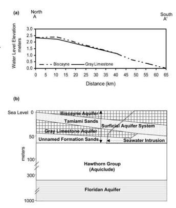
**Figure 2.** Hydrologic cross sections along line A-A' shown on Figure 1. (a) Average water levels measured in this study of the Biscayne and Gray Limestone Aquifers. (b) Hydrogeologic framework beneath Everglades National Park adapted from *Fish and Stewart* [1991] and *Reese and Cunningham* [2000] showing the approximate extent of seawater intrusion in the SAS.
