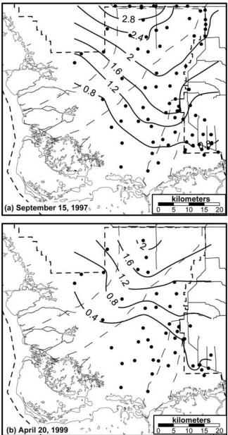
**Figure 4.** Potentiometric contours in meters measured in Everglades National park during the (a) wet season and (b) dry season. Circles represent water level monitoring stations monitored by ENP and the USGS. Data provided courtesy of ENP and USGS.
