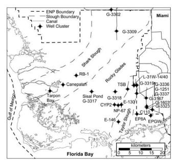
**Figure 3.** Site map showing sampling locations. Circles with cross represent a cluster of one to four groundwater wells screened within the SAS with depths varying from 1.5 to 53.3 m. The deepest well located at G-3319 is finished at the top of the Hawthorn Group at a depth of 73 m.
