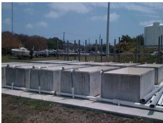
Photo showing layout of twelve, 250-gallon experimental tanks (foreground), salinity mixing and water distribution manifold (wood framed structure) and four, 2000-gallon head tanks (background). Not shown are saltwater pump with connection to Florida Bay, aeration system, and control box (funding SFWMD).
