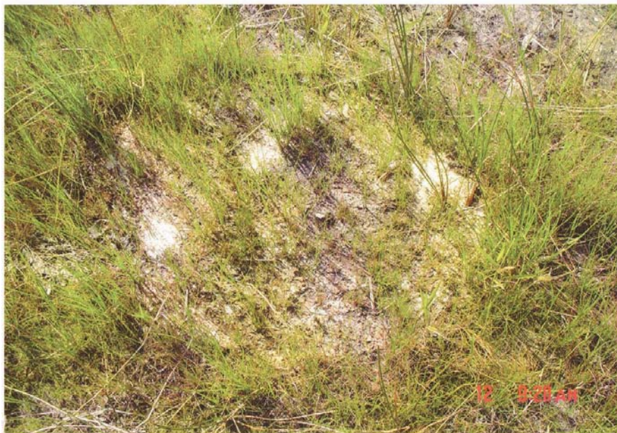
Figure 8.5. Degraded remains of a feldspar marker within a few months of placement. By six months these markers could not be located.
