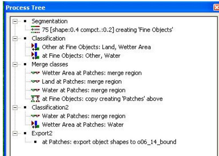
Fig. 1: Process Tree for shoreline creation using Definiens Professional® V5. This tree is used for the Keys. The Process Tree used for coastal areas is similar.
