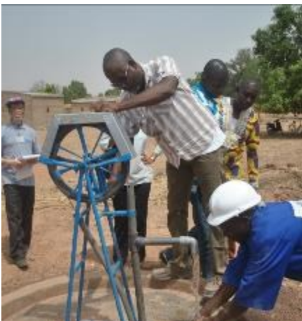
Testing of a rope pump during the visit of the participants to Vipalgo.
