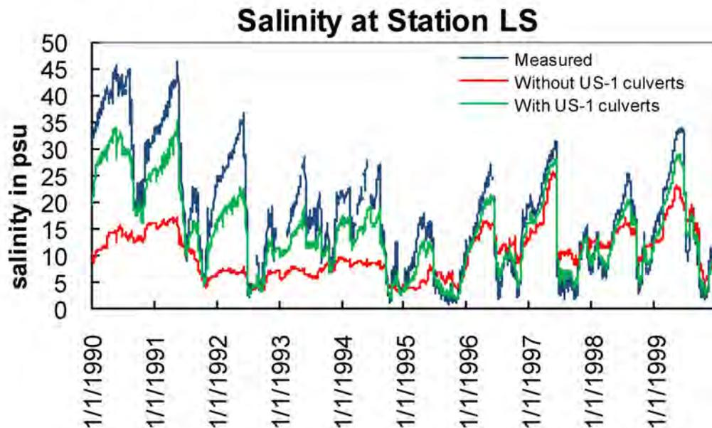
Figure 14. Salinity in Long Sound with addition of culverts under U.S. Highway 1.
