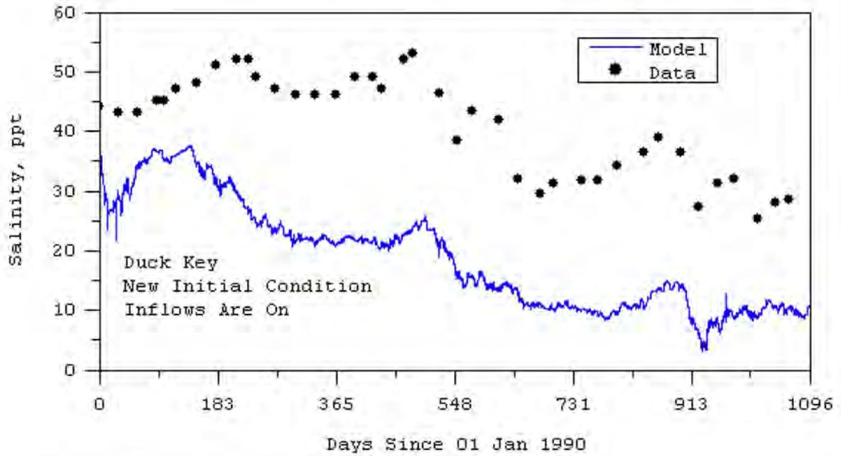
Figure 12: EFDC model test with increased initial salinity.
