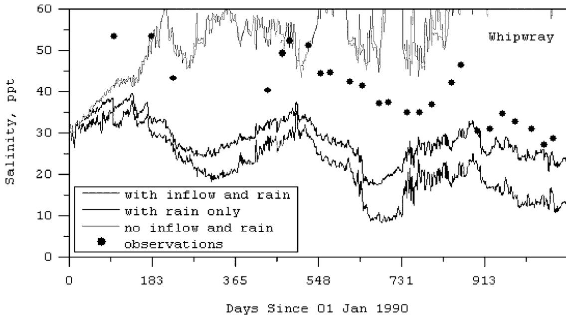
Figure 9: EFDC model test of Alt7R5 with the inflow and rainfall turned off at the Whipray Basin FIU monitoring location.
