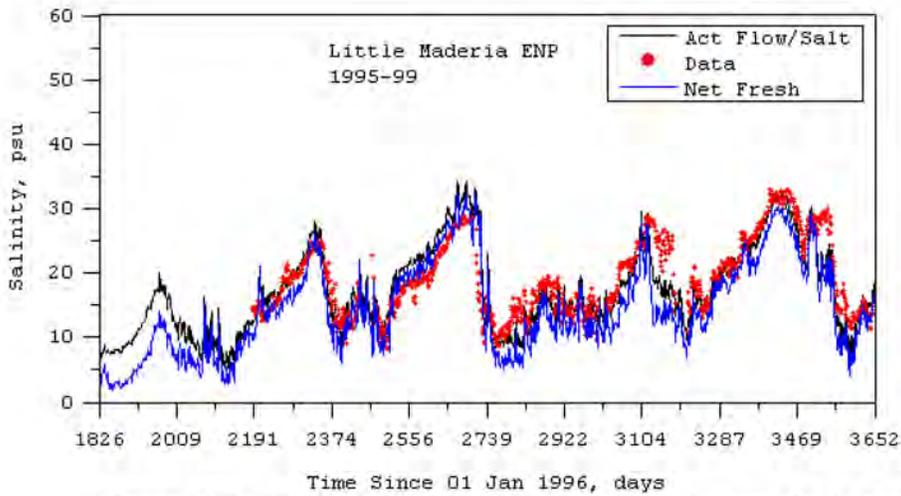
Figure 16B – Little Maderia salinities using two methods to transfer salinity.
