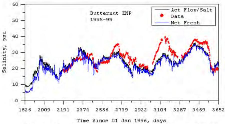
Figure 16C – Butternut Key salinities using two methods to transfer salinity.
