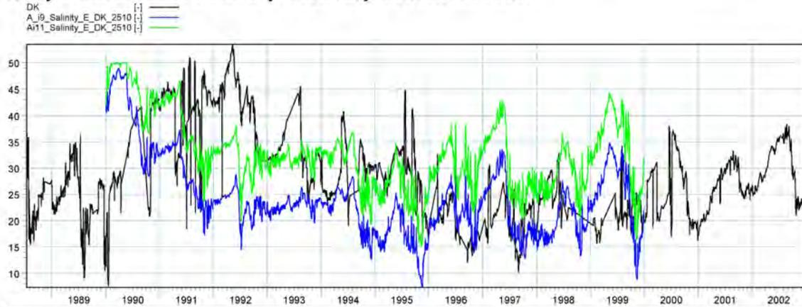
Figure 25: TIME model results at Duck Key showing the differences between runs caused by the increased salinity boundary conditions.
