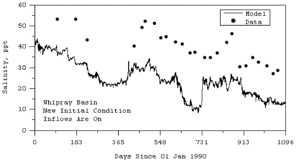
Figure 10: EFDC model test with increased initial salinity from observed data.
