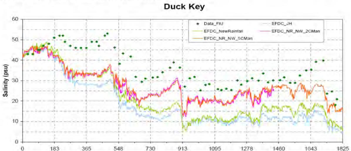
Figure 22: EFDC model results at Duck Key showing the differences between modified input runs.
