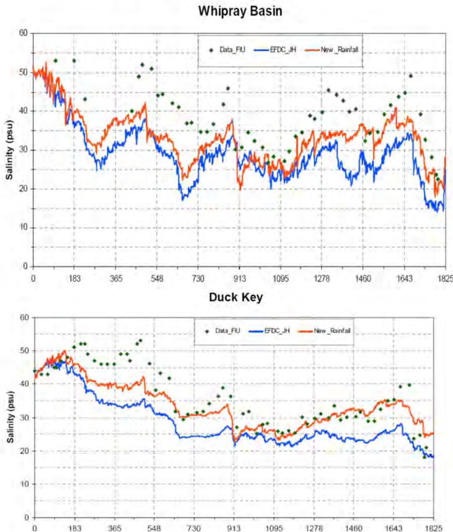
Figure 17: EFDC model test with improved rainfall, increased initial salinity, and updated TIME inputs from the latest testing.
