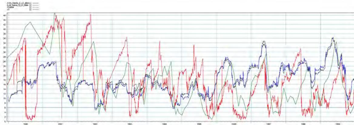
Figure 5: Salinity plot of Long Sound IR with FIU and ENP observed salinity data for the replaced structure input flow test of TIME Alt7R5.
