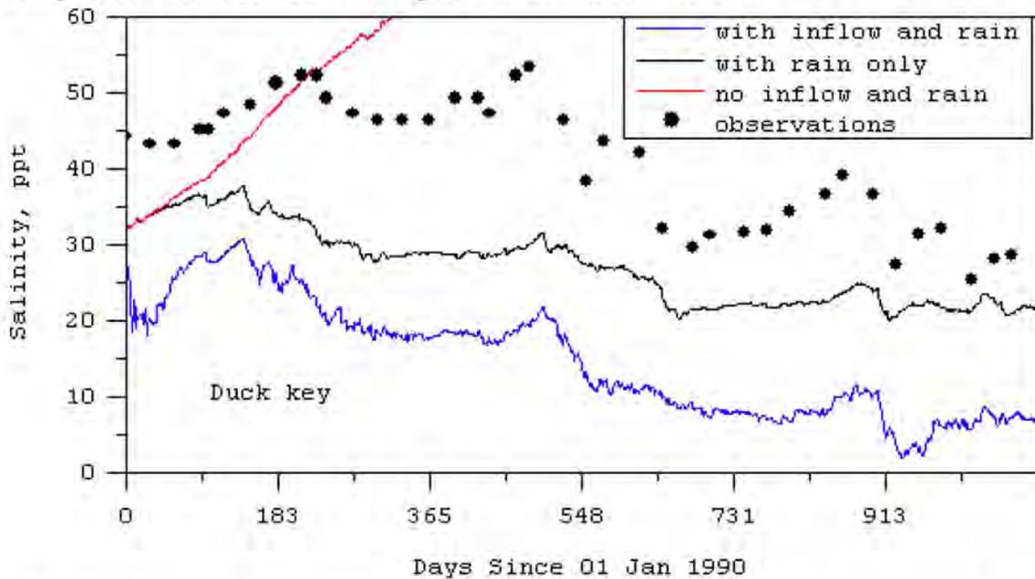
Figure 8: EFDC model test of Alt7R5 with the inflow and rainfall turned off.
