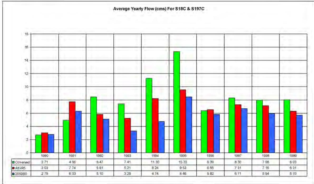
Figure 4: Average yearly combined flows from the S18C and S197 structures for observed, Alt7R5 and 2050B0.
