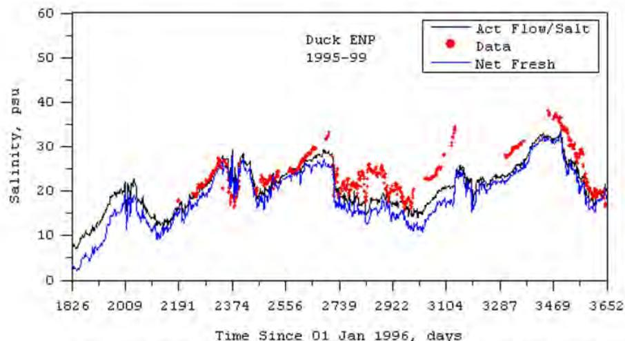
Figure 16A – Duck Key salinities using two methods to transfer salinity.
