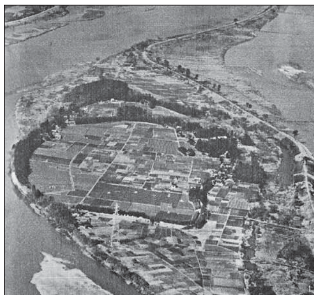
Figure 2. The Waju protects the community from floods (Photo by Iwanami Co., Ltd., 1956)
