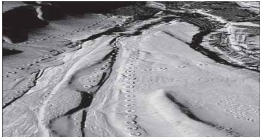
Figure 2. Aerial image of vertical wells in Turpan area of China. Source: www.sunnynchina.com
