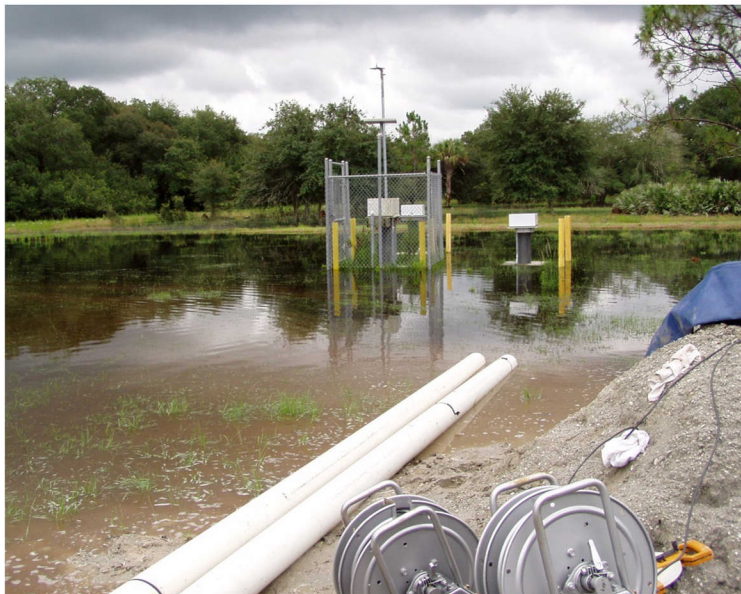
Figure 17. Wet site conditions during step-drawdown testing.
