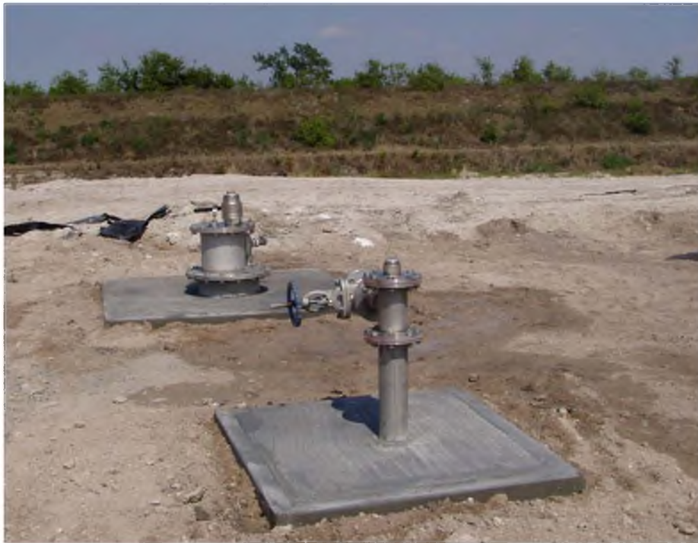
Floridan Aquifer System Monitor Well MF-40 and Intermediate Confining Unit Monitor Well MH-40
