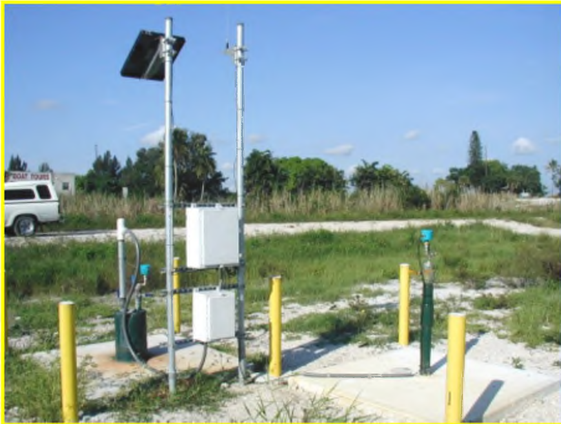
Cover Photo: W. Hillsboro Canal Tri-zone Floridan Aquifer System Monitor Well with Recorder and Telemetry
