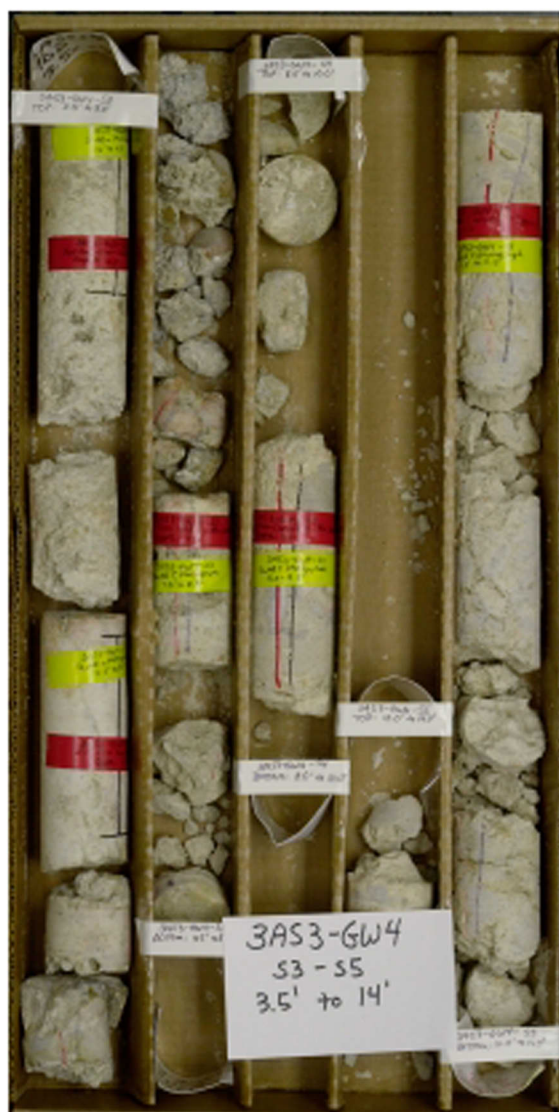
Figure B-5. Core from Well 3AS3-GW4, 3.5 to 14 ft below Peat
