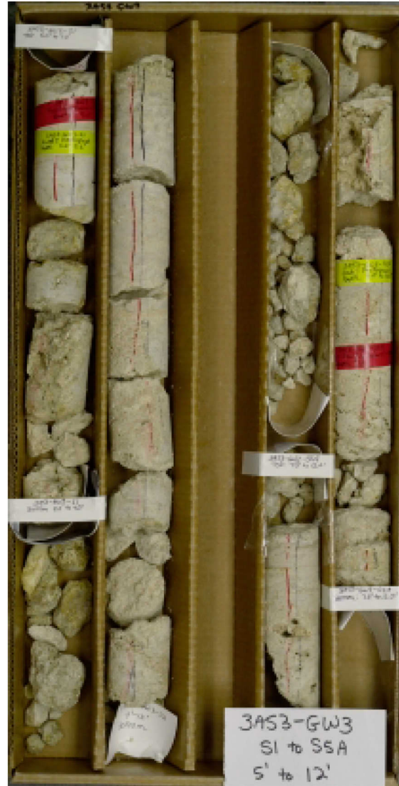
Figure B-4. Core from Well 3AS3-GW3, 5 to 12 ft below Peat
