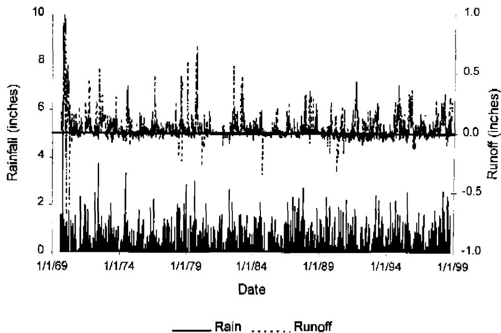
Figure 40. Temporal results for rainfall and runoff in S65D sub-basin.
