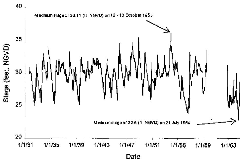
Figure 29. Daily stage for monitoring station C38.BAS.
