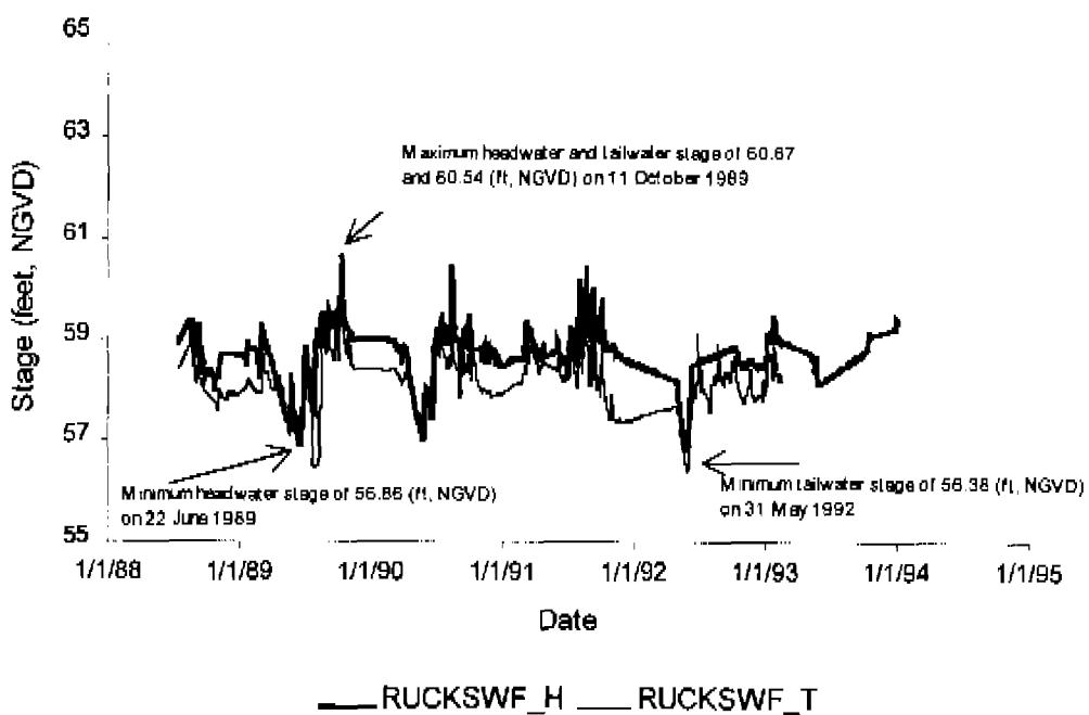
Figure 24. Daily stage for monitoring station RUCKSWF.
