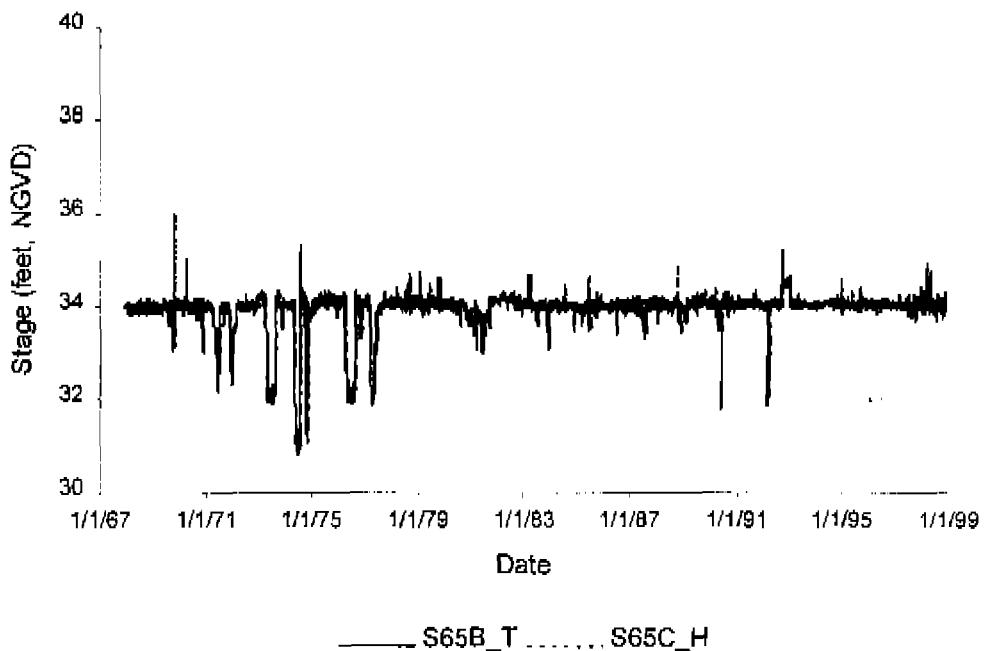
Figure 15. Daily stage for monitoring stations S65B\_T and S65C\_H.
