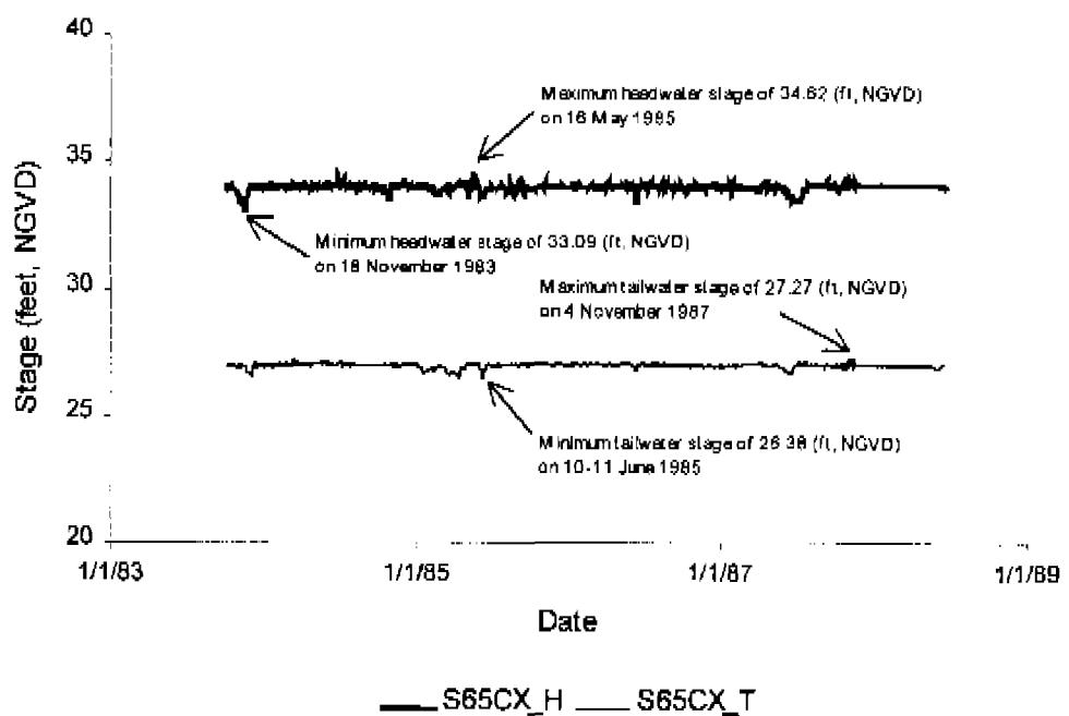
Figure 13. Daily stage for monitoring station S65CX.
