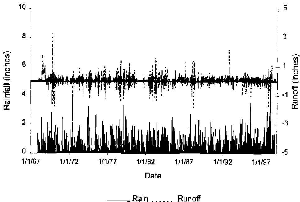
Figure 37. Temporal results for rainfall and runoff in S65C sub-basin.
