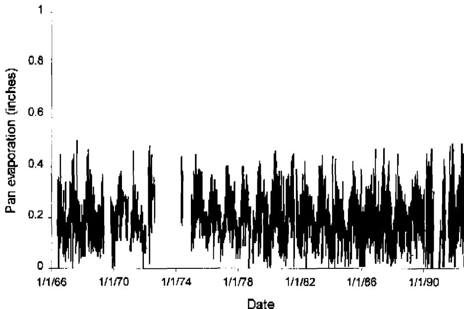
Figure 5. Daily pan evaporation results for station S65C\_E.
