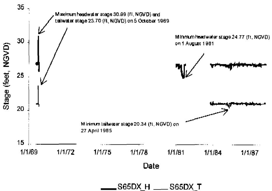
Figure 30. Daily stage for monitoring station S65DX.
