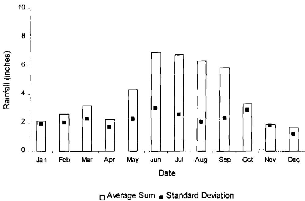
Figure 7. Mean monthly areal rainfall and standard deviation in S65C sub-basin for years 1957 – 1997.
