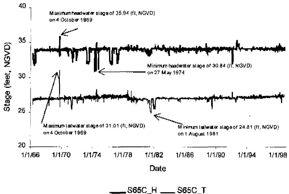
Figure 14. Daily stage for monitoring station S65C.
