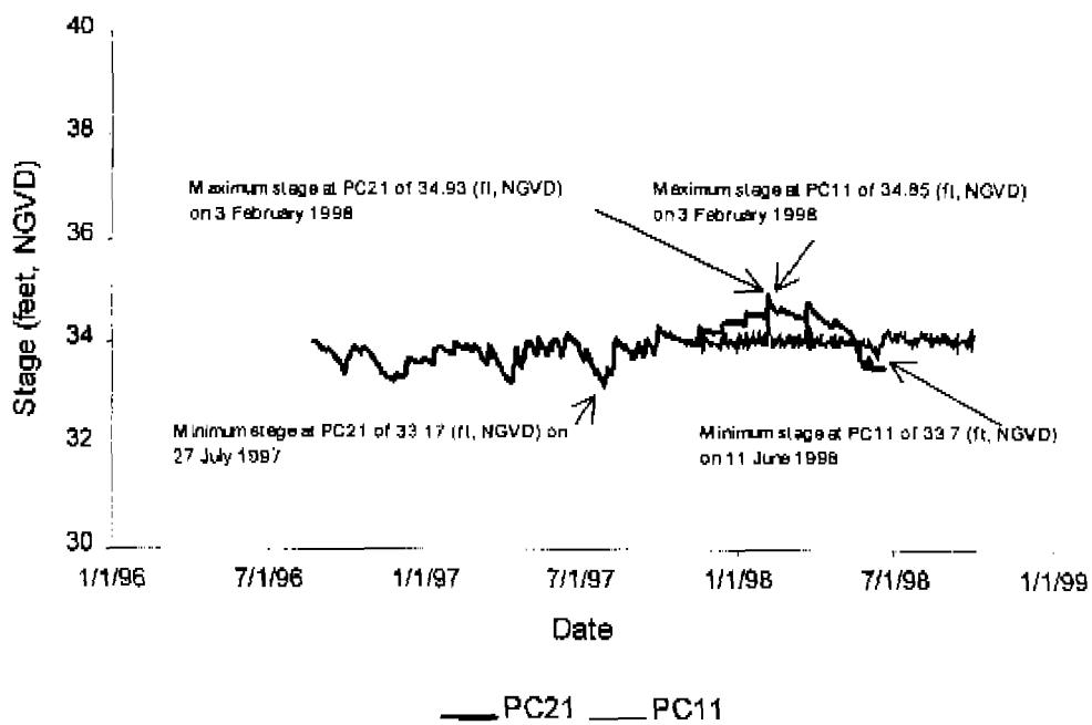
Figure 11. Daily stage for monitoring stations PC21 and PC11.
