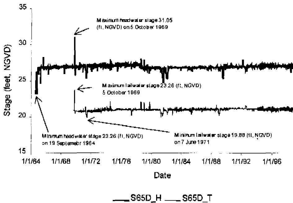
Figure 31. Daily stage for monitoring station S65D.
