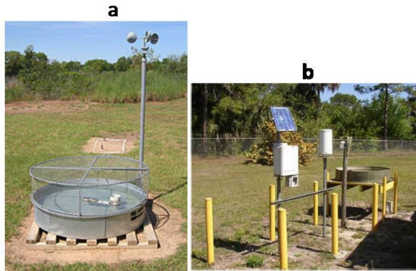
Figure 3. Evaporation pan with elevated bird guard (a) and with elevated platform (b).
