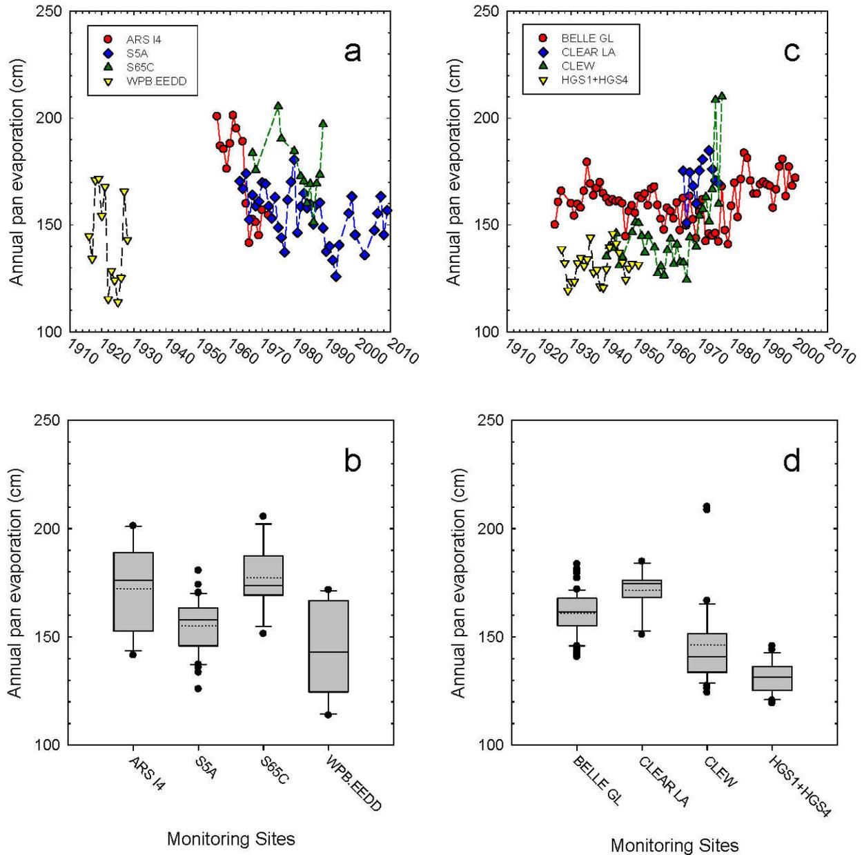
Figure 5. Evaporation pans sites with decreasing (a, b) and increasing (c, d) trends and comparative statistics (box plots). Dashed lines on the box plots indicate means and solid lines indicate medians of the pan evaporation data for each site.
