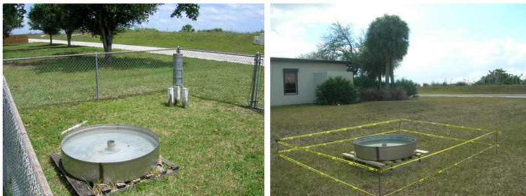
Figure 4 Relocation of an evaporation pan site in South Florida.
