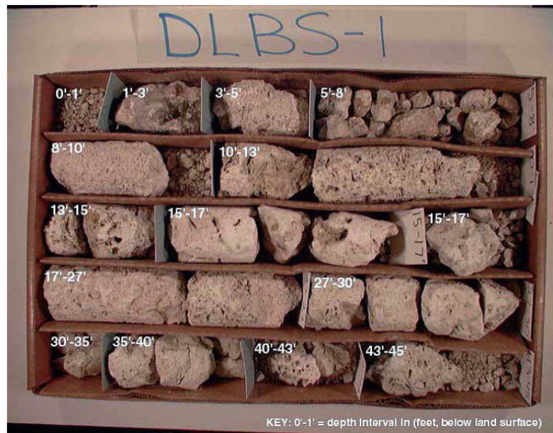
Figure 5. Photograph of DLBS-1 Core where Dense Limestone Zone was Identified at 5-8 feet bls
