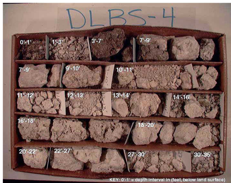
Figure 8. Photograph of DLBS-4 Core where Dense Limestone Zone was Identified at 10-11 feet bls
