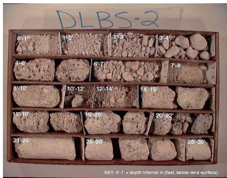
Figure 6. Photograph of DLBS-2 Core where Dense Limestone Zone was Identified at 10-14 feet bls
