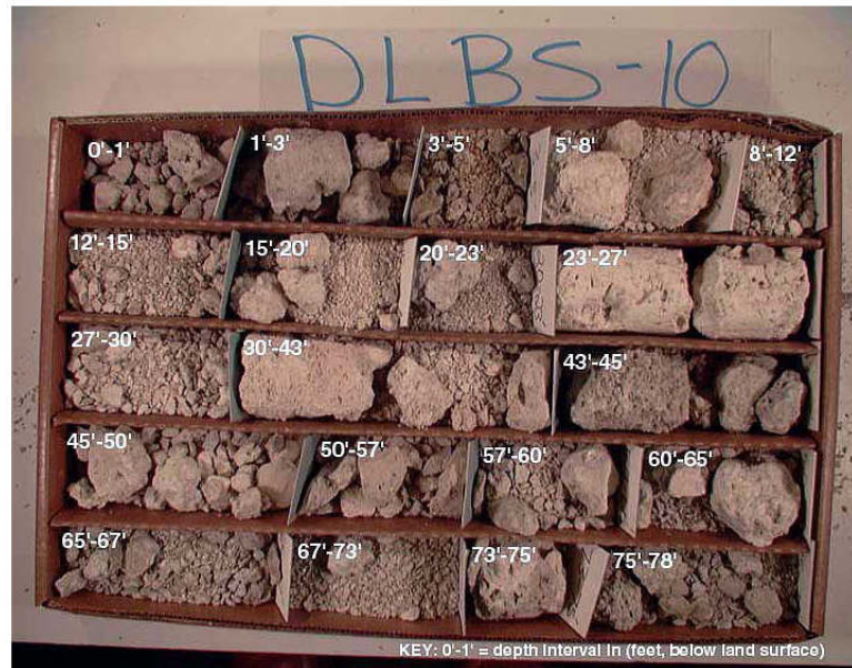
Figure 13. Photograph of DLBS-10 Core where Dense Limestone Zone was Identified at 3-5 feet bls
