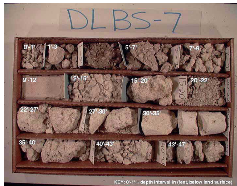
Figure 10. Photograph of DLBS-7 Core where Dense Limestone Zone was Identified at 15-20 feet bls
