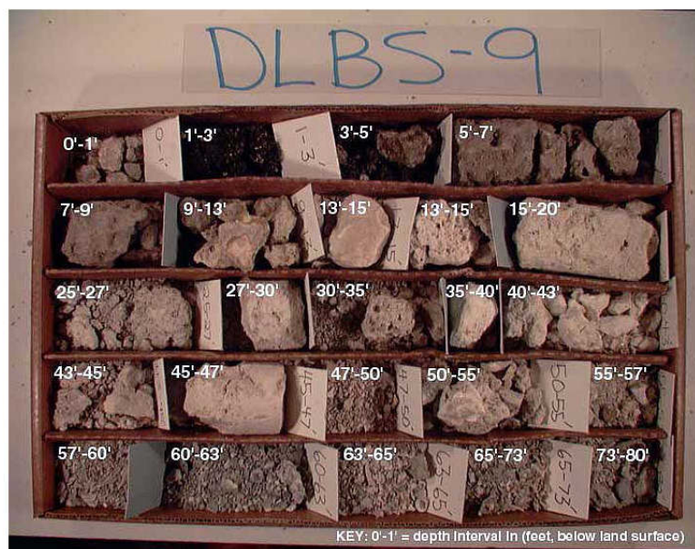
Figure 12. Photograph of DLBS-9 Core where Dense Limestone Zone was Identified at 9-15 feet bls
