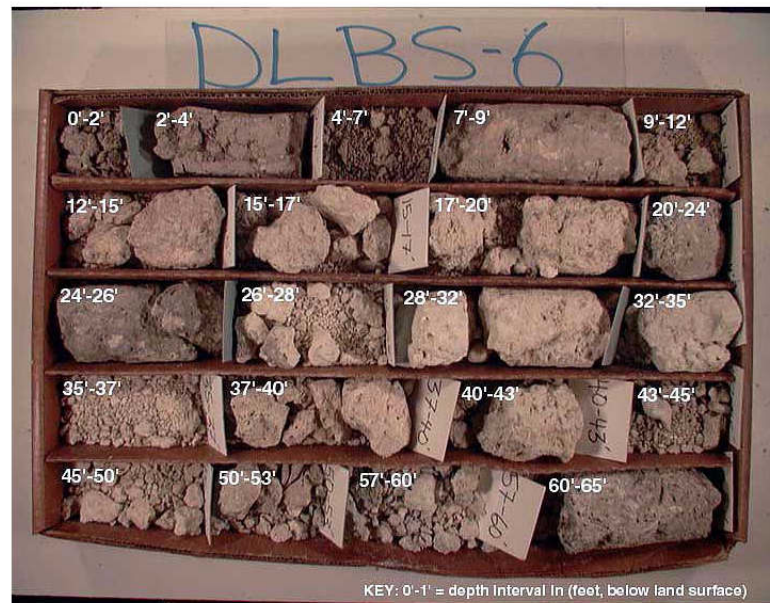
Figure 9. Photograph of DLBS-6 Core where Dense Limestone Zone was Possibly Identified at 15-17 feet bls
