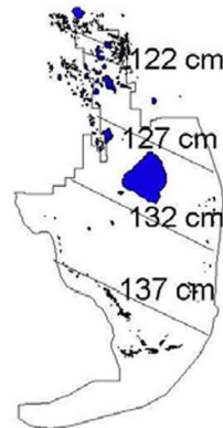
Figure 5. Estimated potential evapotranspiration isohyetal lines for the South Florida Water Management District area.
