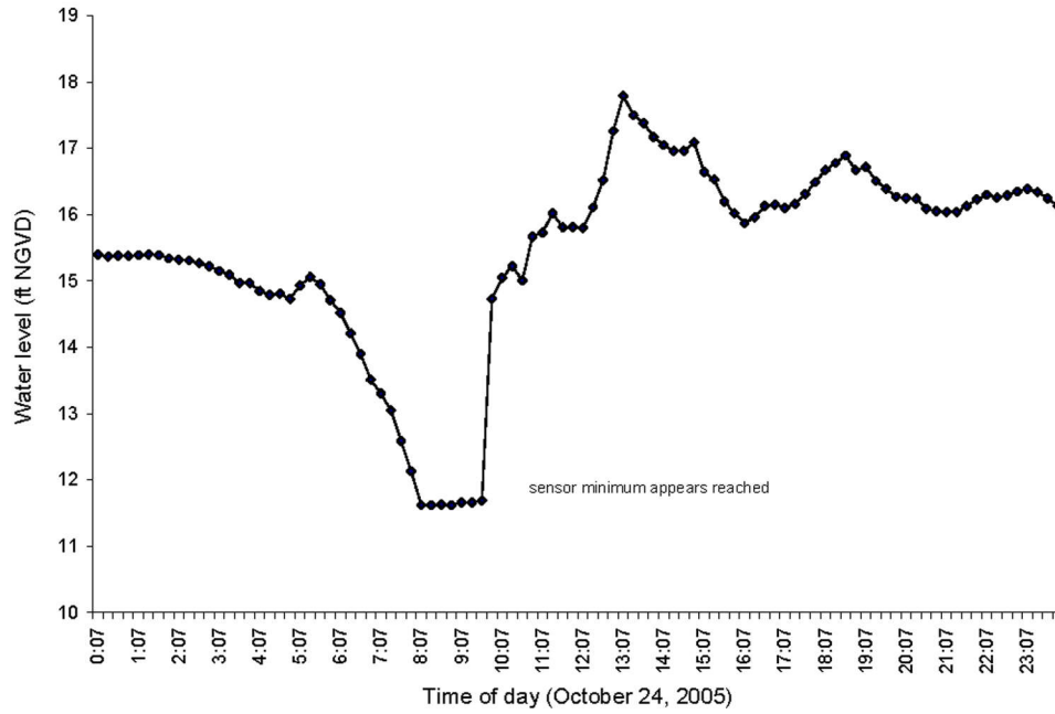
Figure 50. Lake Okeechobee water level changes at the S-135 structure during Hurricane Wilma.
