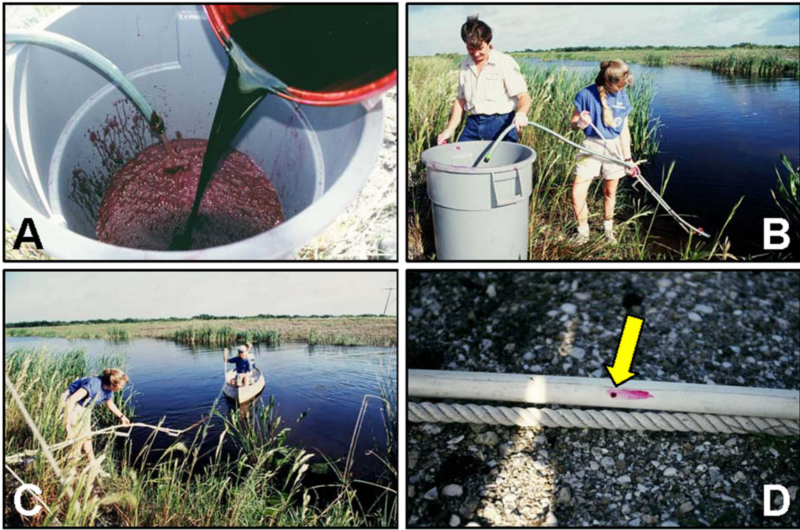
Figure 2. Preparations for releasing dye tracer into the Everglades Nutrient Removal Project, October 1994. Panel A: diluting the stock Rhodaine WT dye solution in the holding tank; Panel B: attaching diffuser pipe apparatus to the holding tank; Panel C: positioning diffuser pipe across the distribution canal downstream of the Inflow Pump Station; Panel D: close-up of a port in the diffuser pipe.
