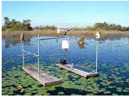
Figure 4. Bowen ratio-energy balance instrumentation on in Loxahatchee National Wildlife Refuge, Site 3 (German, 2000).
