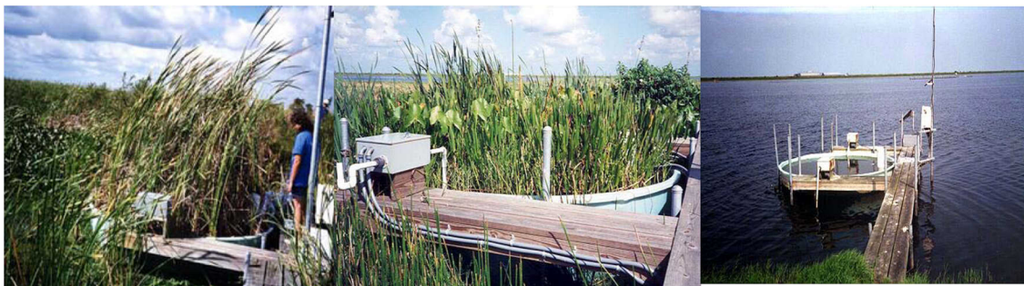
Figure 2. Cattail, mixed vegetation, and open water lysimeters in the Everglades Nutrient Removal constructed wetland.
