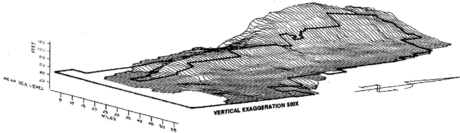
**Figure 33** THREE-DIMENSIONAL REPRESENTATION OF THE POTENTIOMETRIC SURFACE OF THE FLORIDAN AQUIFER SYSTEM, MAY 1981
