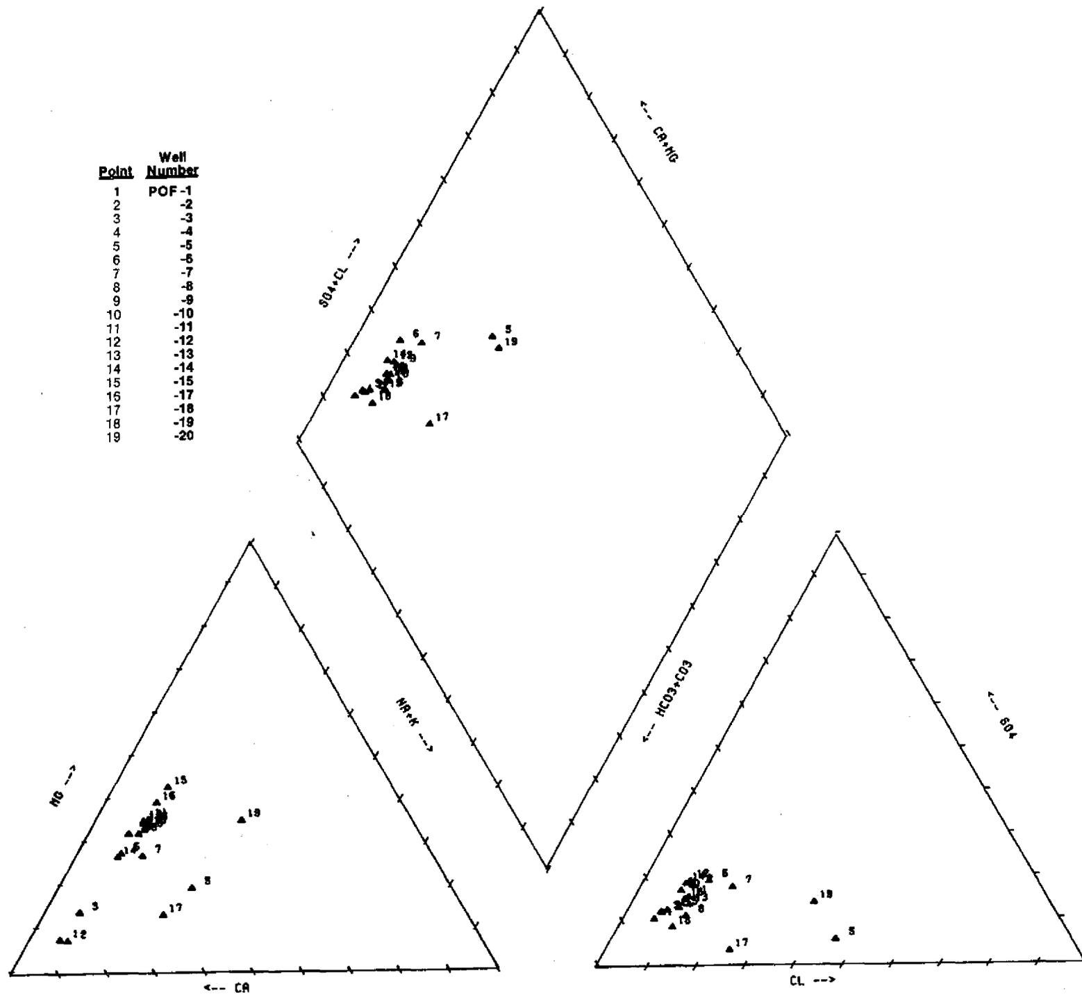
Figure 58 PIPER TRILINEAR DIAGRAM FOR POLK COUNTY
