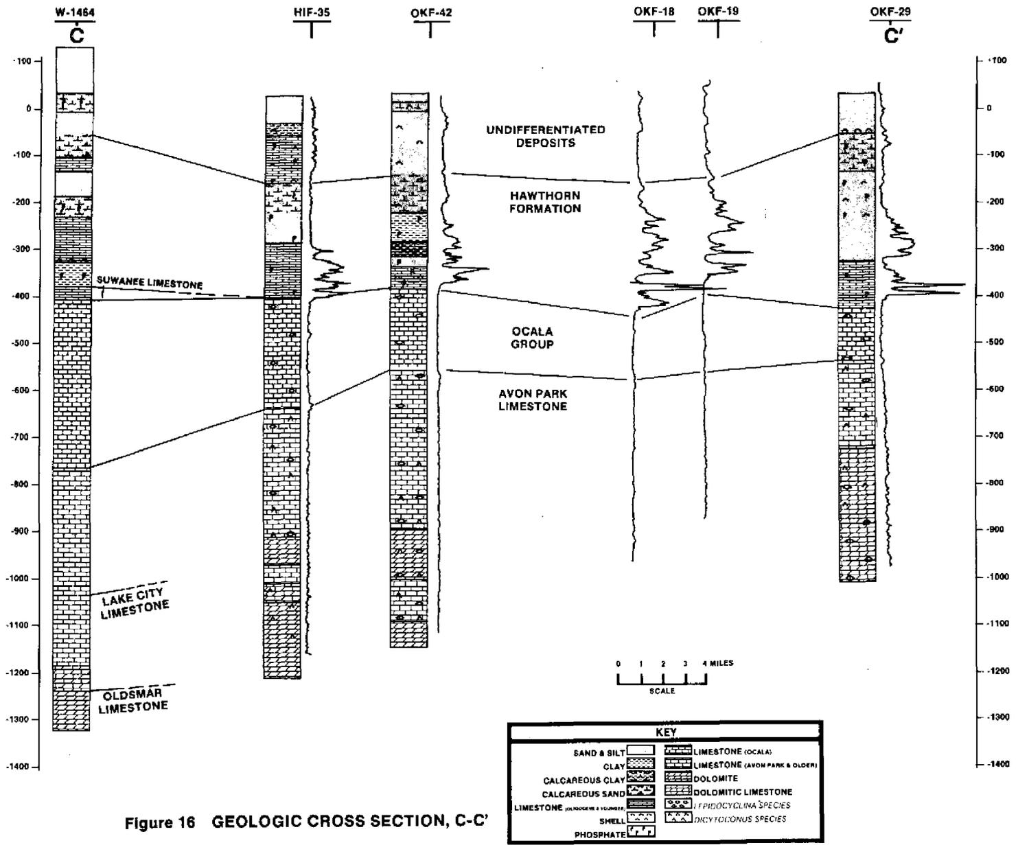
Figure 16 GEOLOGIC CROSS SECTION, C-C'
