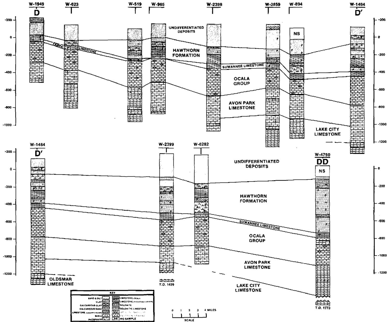
Figure 17 GEOLOGIC CROSS SECTION, D-DD
