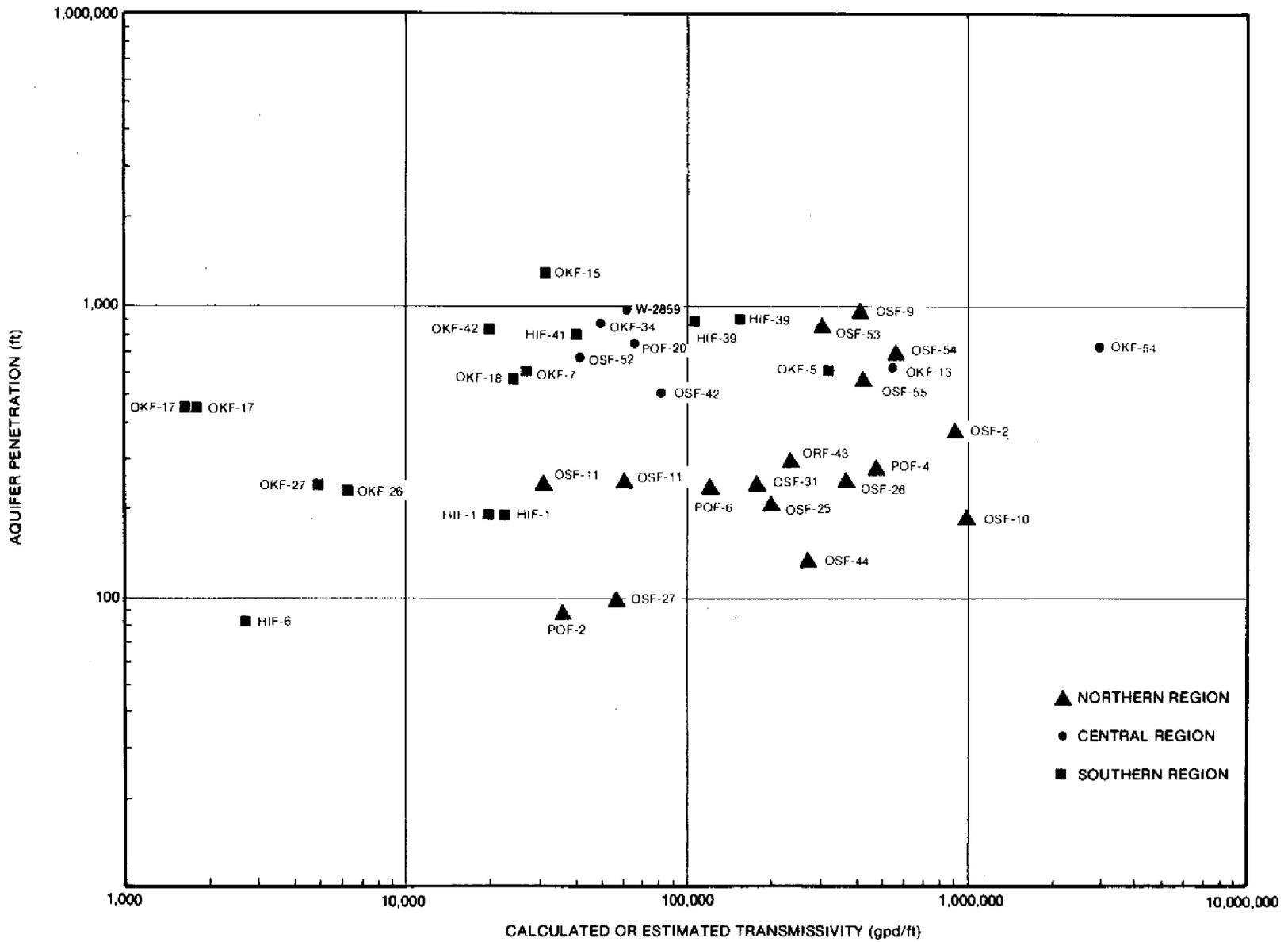
**Figure 69 CALCULATED OR ESTIMATED TRANSMISSIVITY VERSUS AQUIFER PENETRATION FOR SELECTED WELLS**
