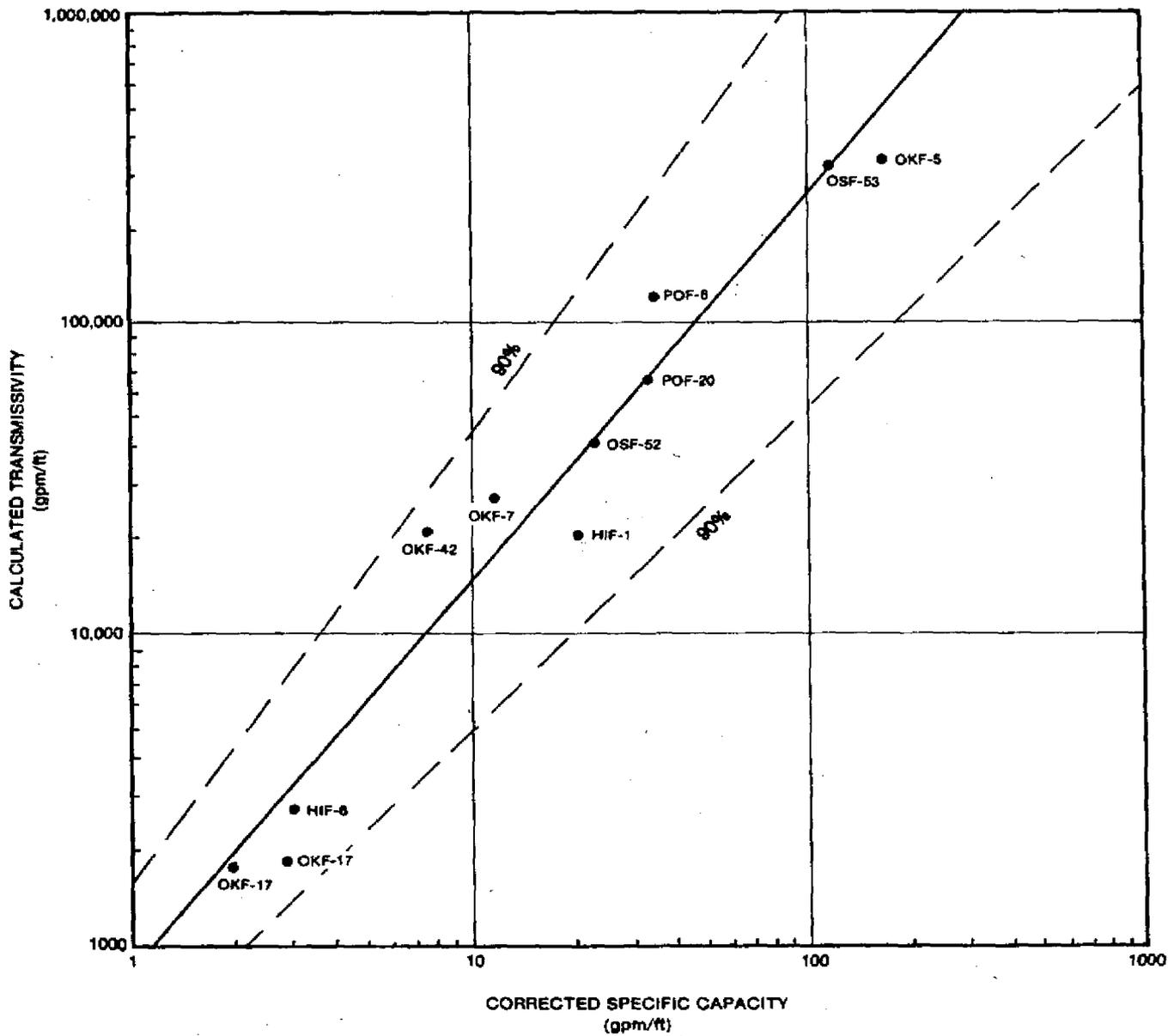
**Figure 68 CORRECTED SPECIFIC CAPACITY VERSUS CALCULATED TRANSMISSIVITY FROM RESIDUAL RECOVERY ANALYSIS FOR SELECTED WELLS**
