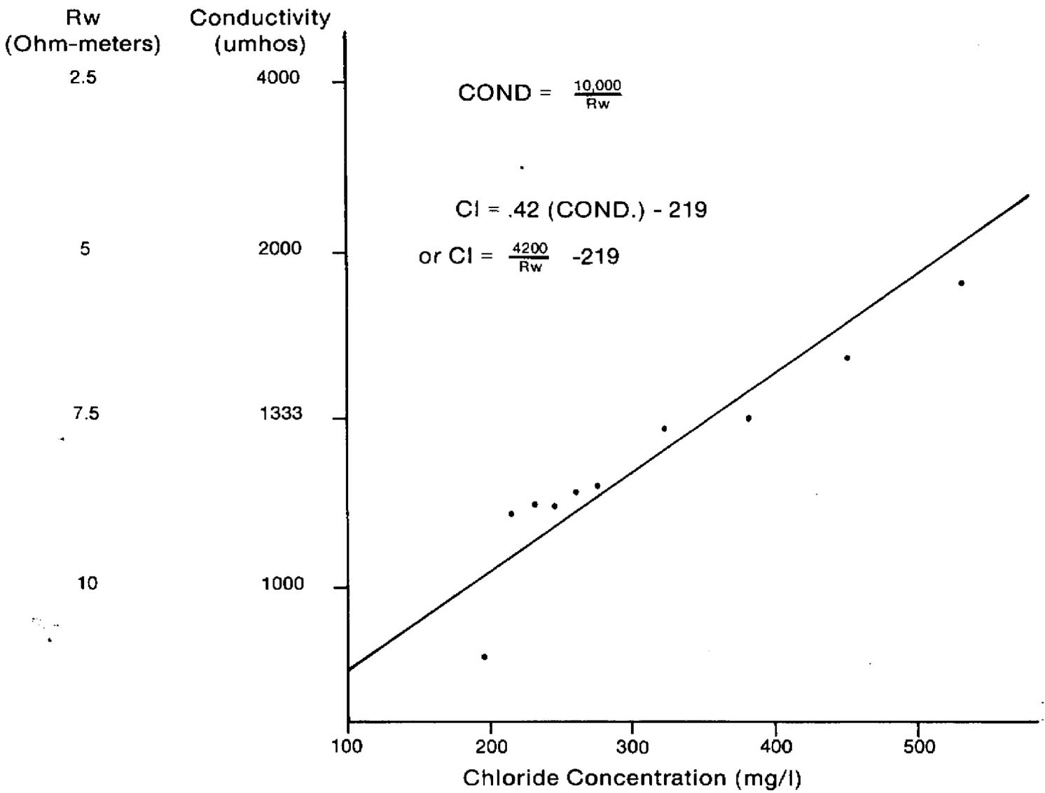
**Figure 66 CHLORIDE CONCENTRATION VERSUS FLUID RESISTIVITY, WELL HIF-38**
