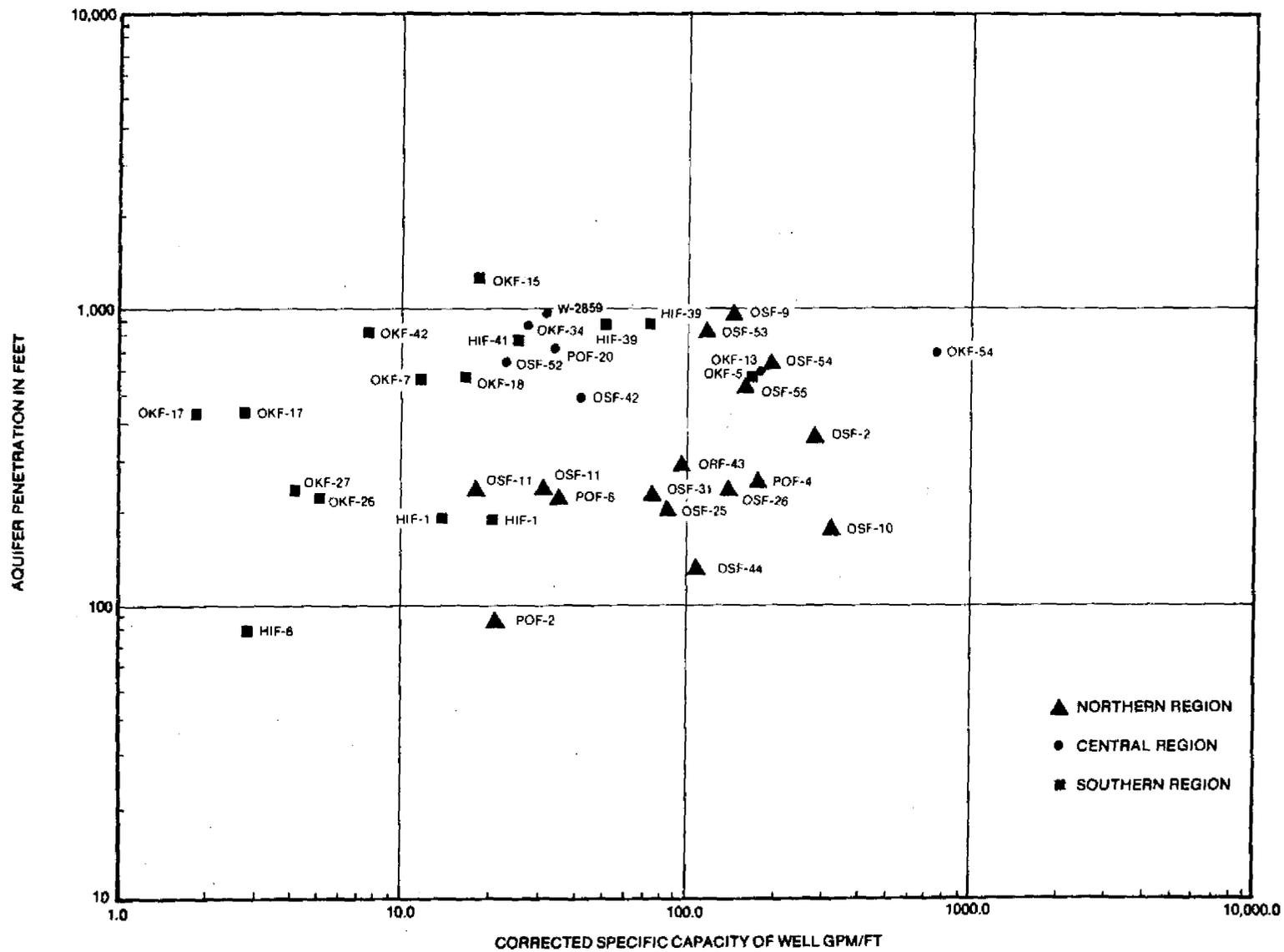
Figure 72 CORRECTED SPECIFIC CAPACITY VERSUS AQUIFER PENETRATION FOR SELECTED WELLS
