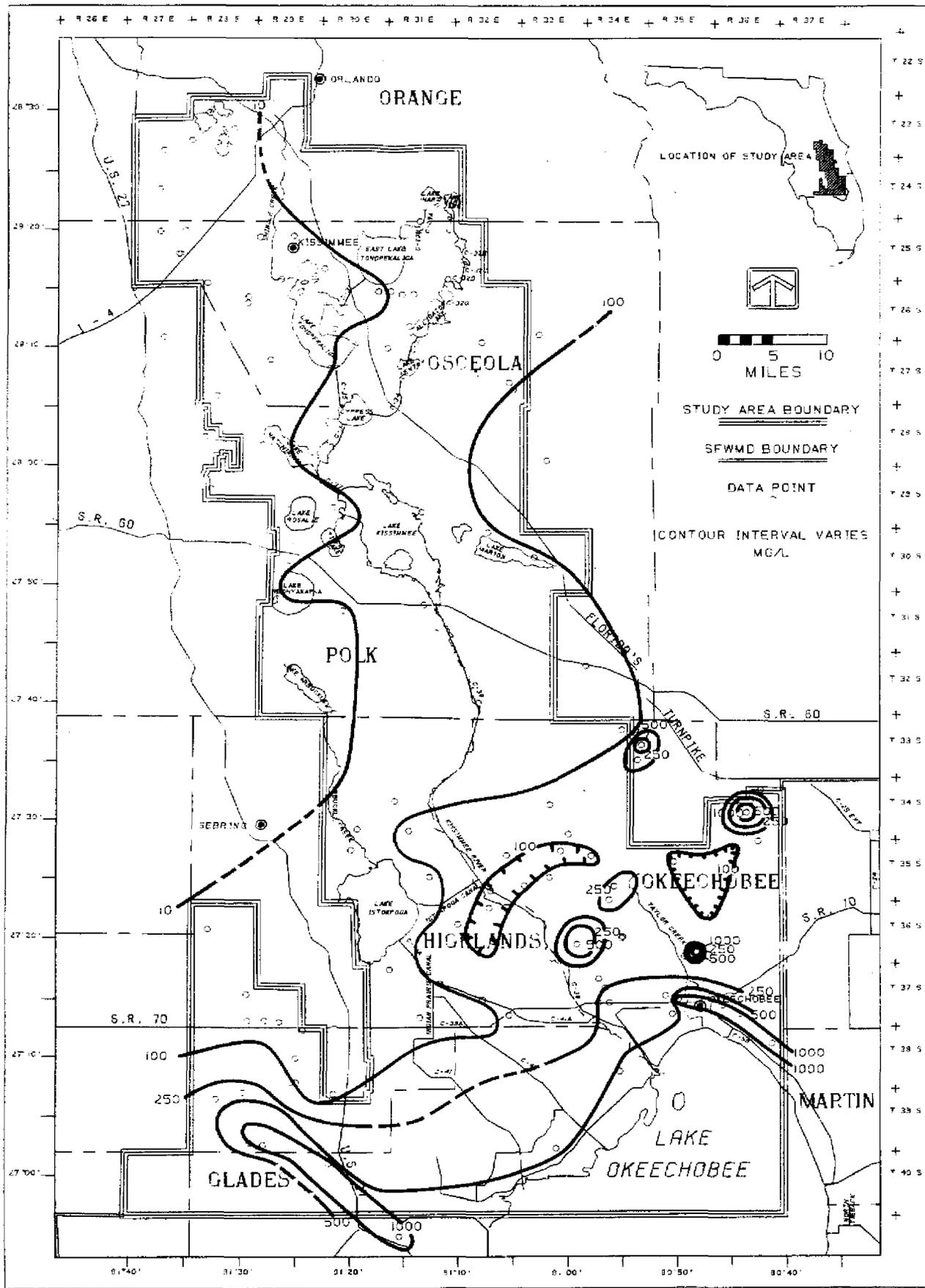
**Figure 48 AVERAGE WELLHEAD CHLORIDE CONCENTRATION, FLORIDAN AQUIFER SYSTEM**
