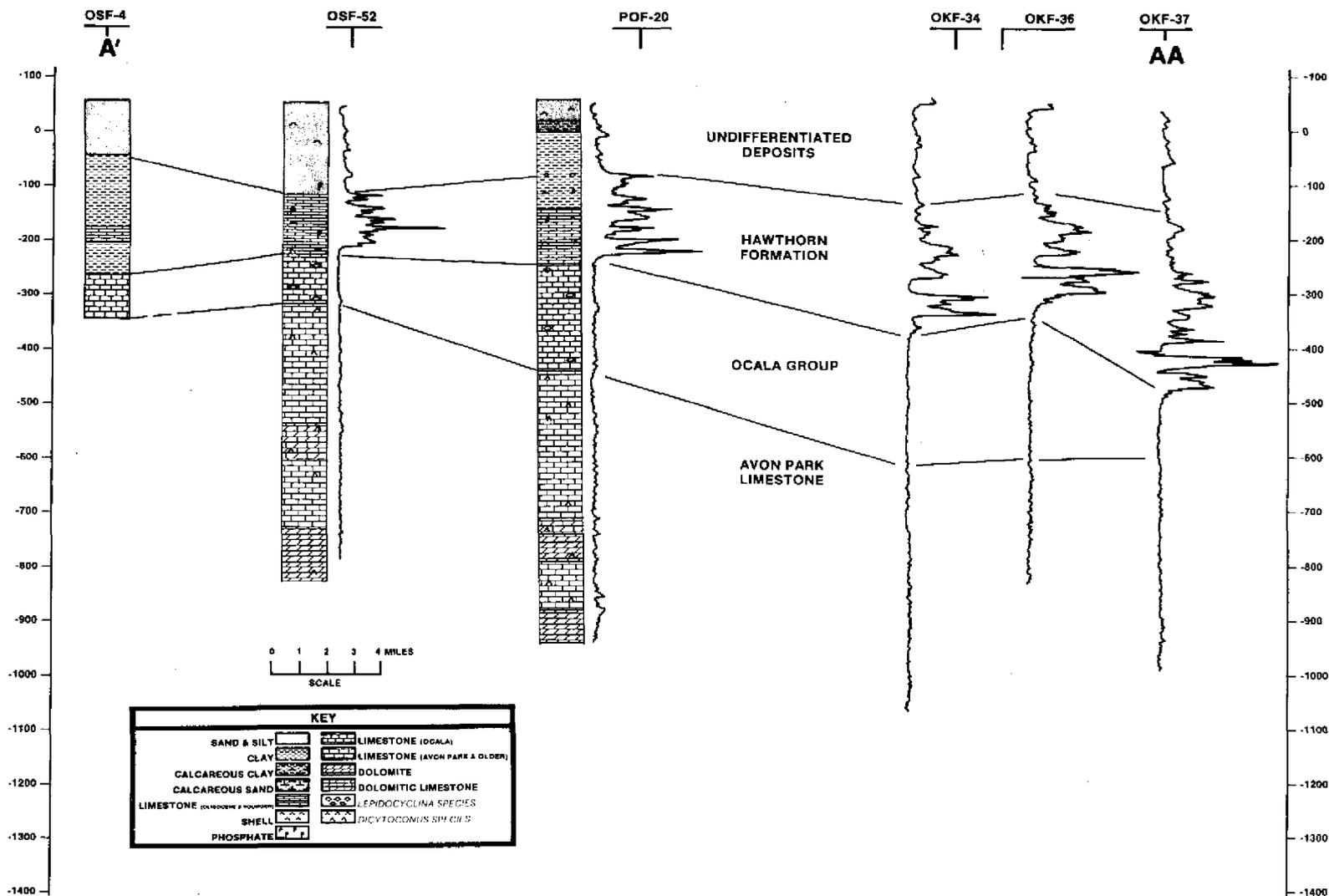
Figure 12 GEOLOGIC CROSS SECTION, A'-AA
