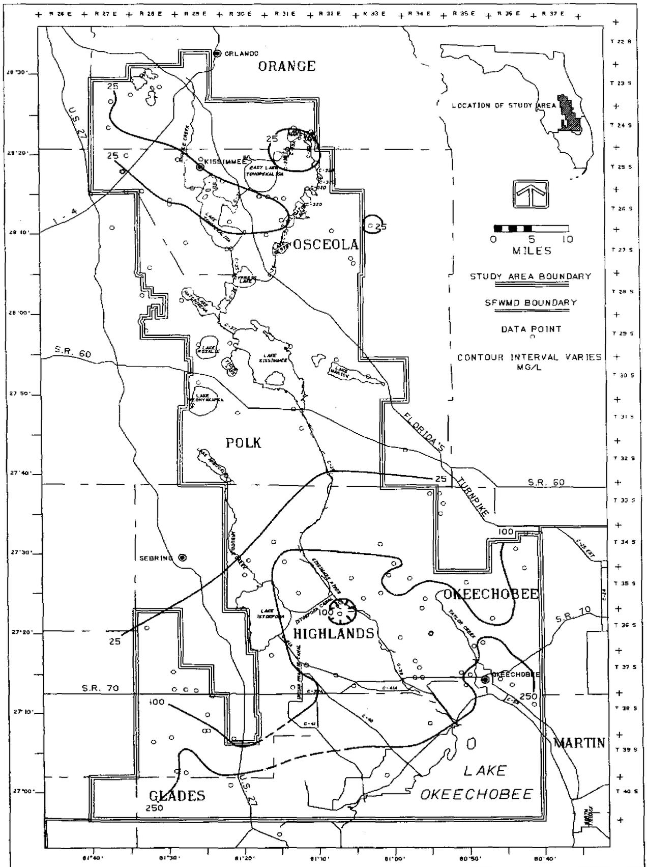
Figure 53 AVERAGE WELLHEAD SULFATE CONCENTRATION, FLORIDAN AQUIFER SYSTEM
