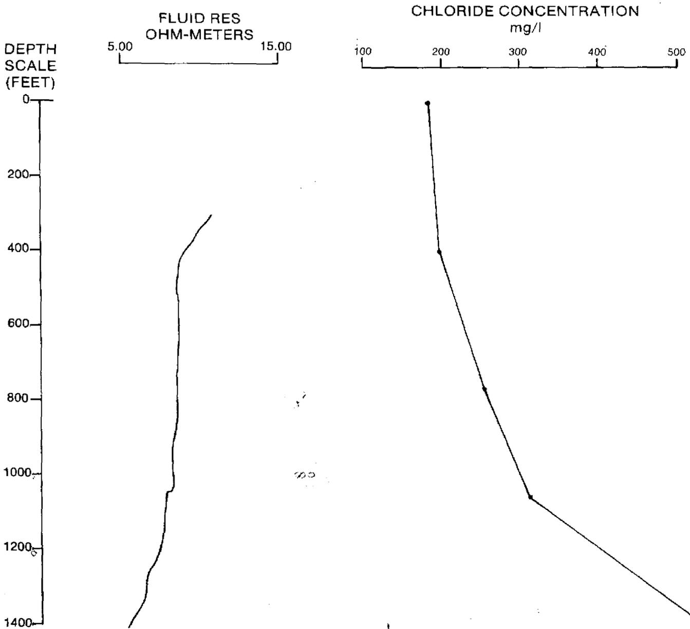
**Figure 65 FLUID RESISTIVITY AND CHLORIDE CONCENTRATION WITH DEPTH, WELL HIF-38**
