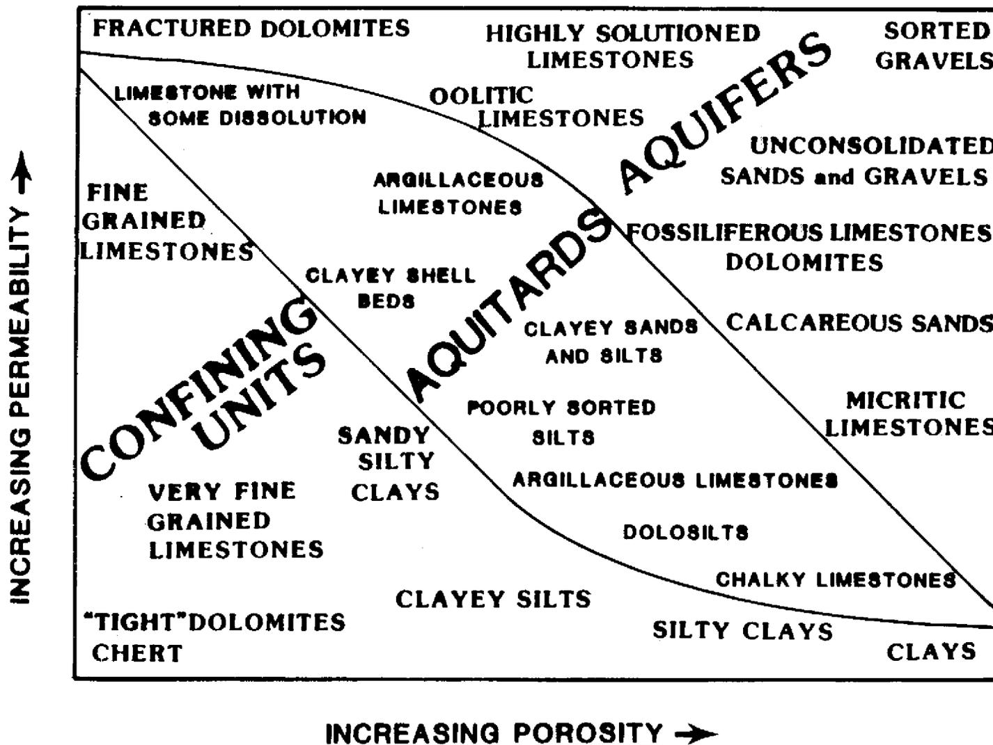
**Figure 18 PERMEABILITY AND POROSITY OF VARIOUS ROCK TYPES (FROM KWADER, 1983, WITH PERMISSION)**
