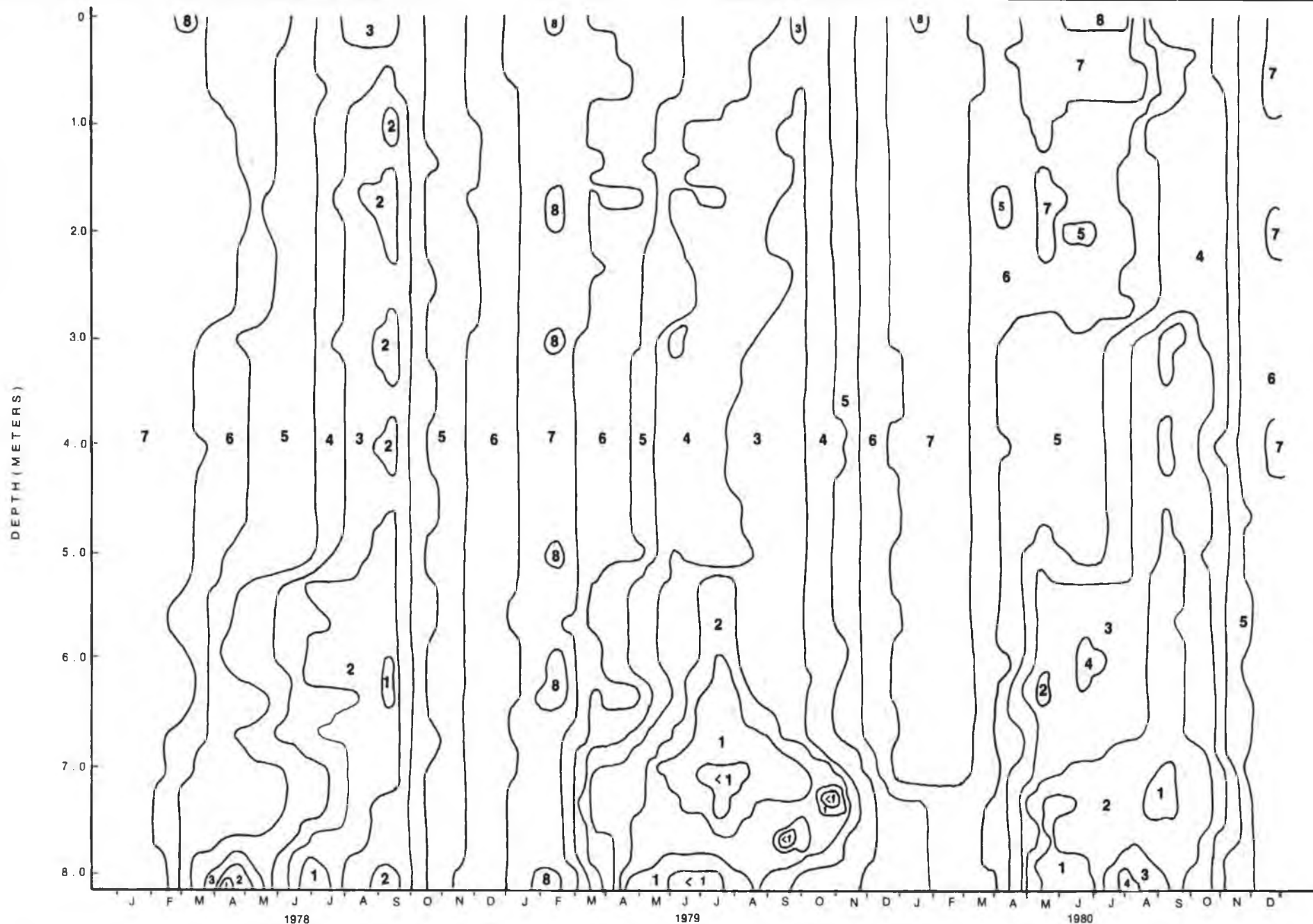
Figure 34 DEPTH-TIME DIAGRAM OF ISOPLETHS OF DISSOLVED OXYGEN CONCENTRATION IN MILLIGRAMS • LITER -1 AT STATION CR-30.4 WEST BASIN 1978-1980
