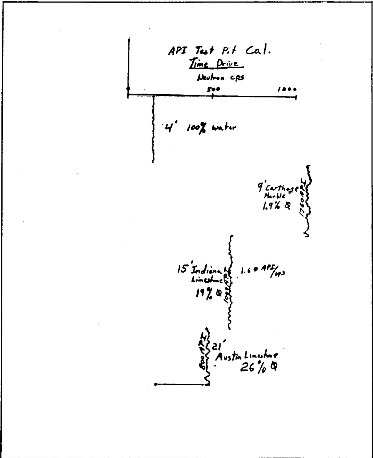
Figure 13 - Neutron porosity responses with the probe stationary at the center of each test pit media.
