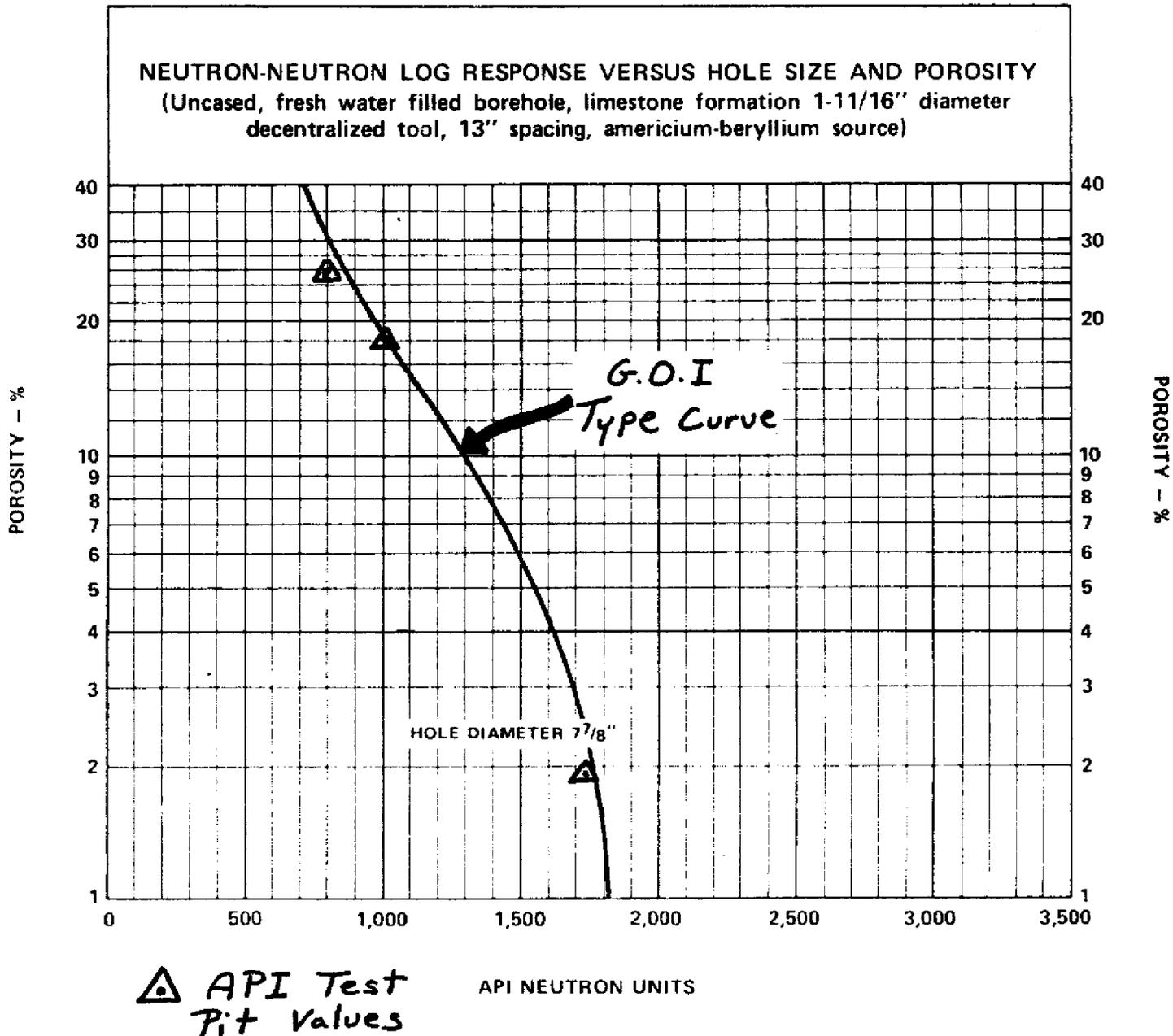
Figure 15 - Type neutron log response with API Test Pit measurements superimposed on curve (modified from GOI, 1977).
