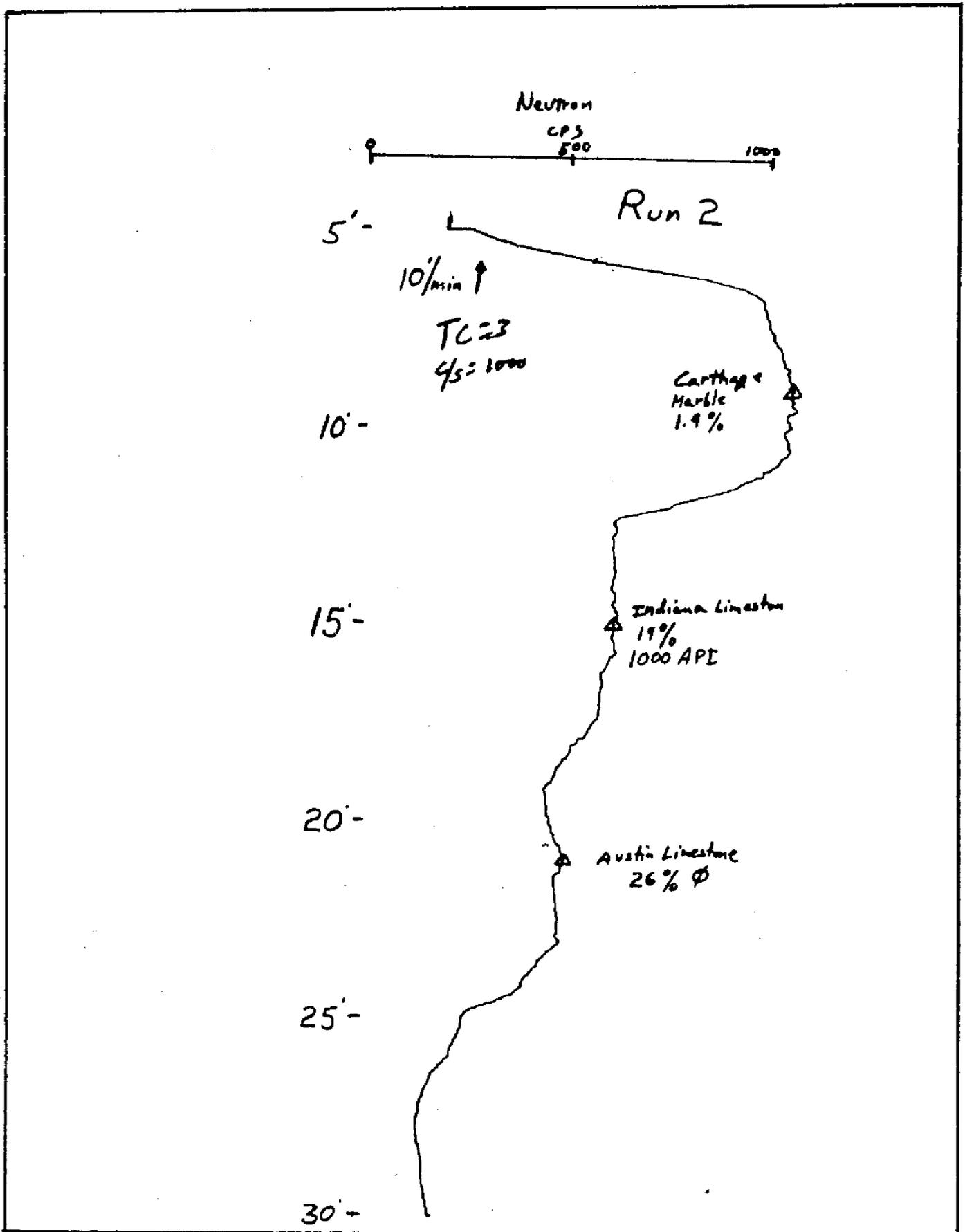
Figure 12 - Neutron porosity test Run #2 in the API Test Pit.
