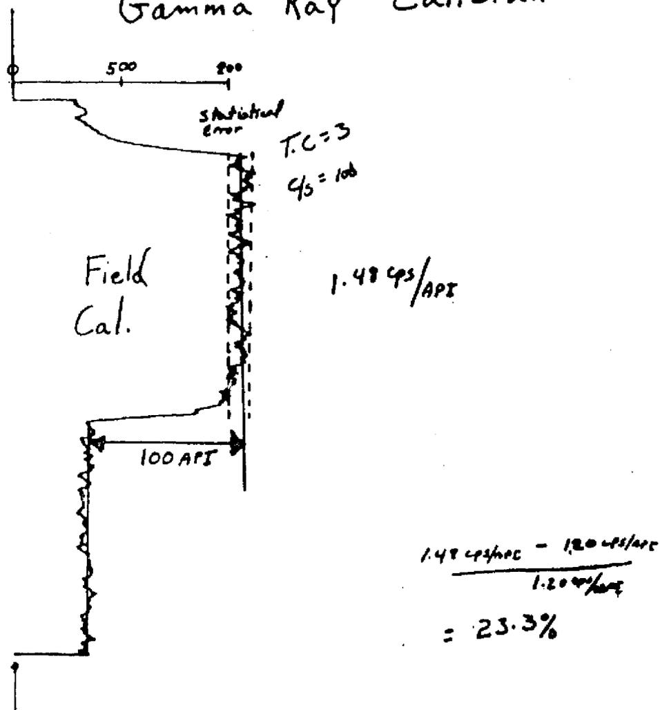
Figure 10 - Natural gamma ray calibration using the GOI gamma ray field calibrator.
