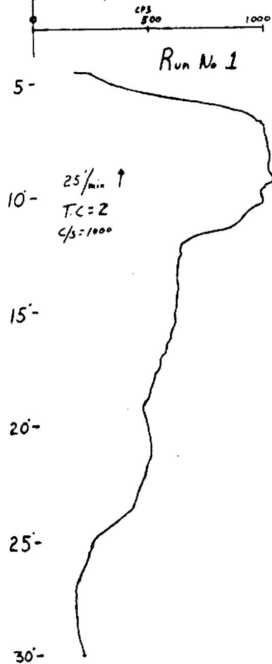
Figure 11 - Neutron porosity test Run #1 in the API Test Pit.
