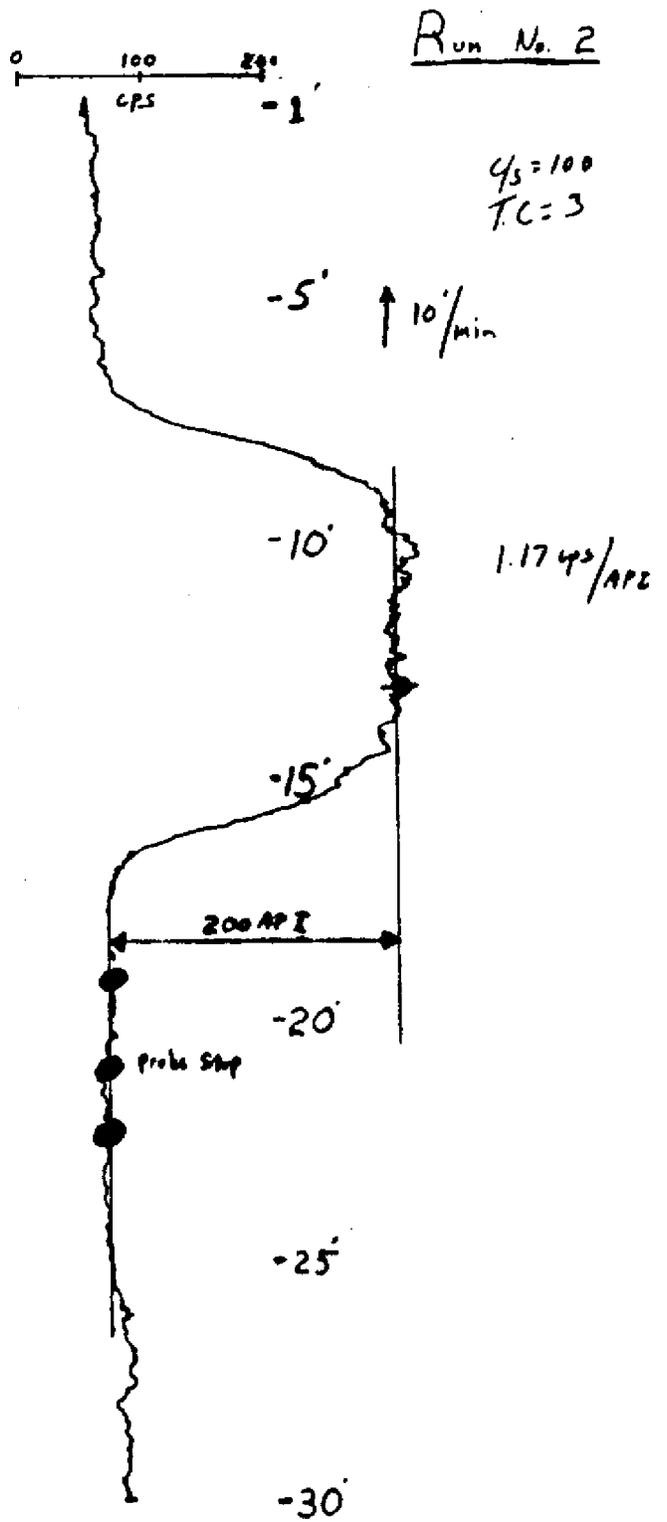
Figure 9 - Natural gamma ray Run #2 in the gamma ray API Test Pit, University of Houston.
