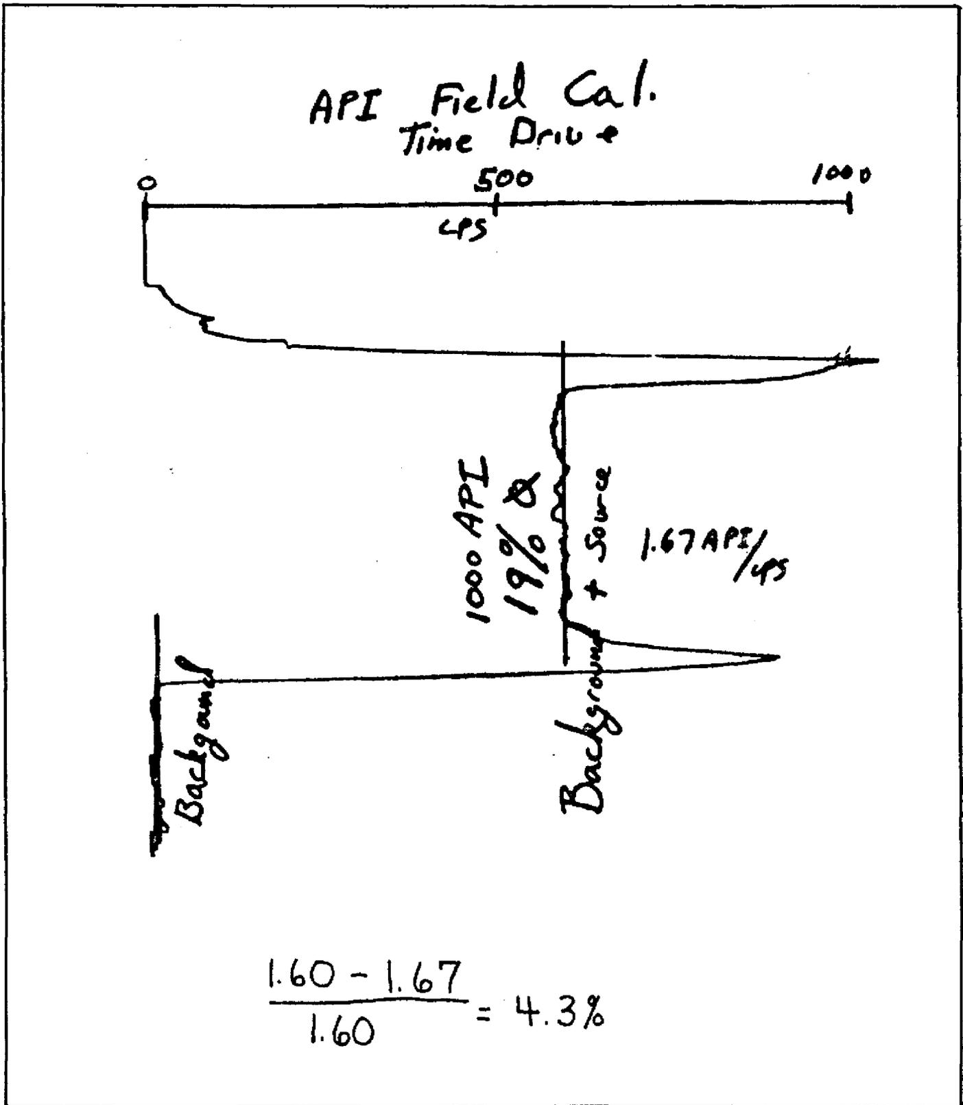
Figure 14 - Neutron porosity calibration using the GOI field calibrator.
