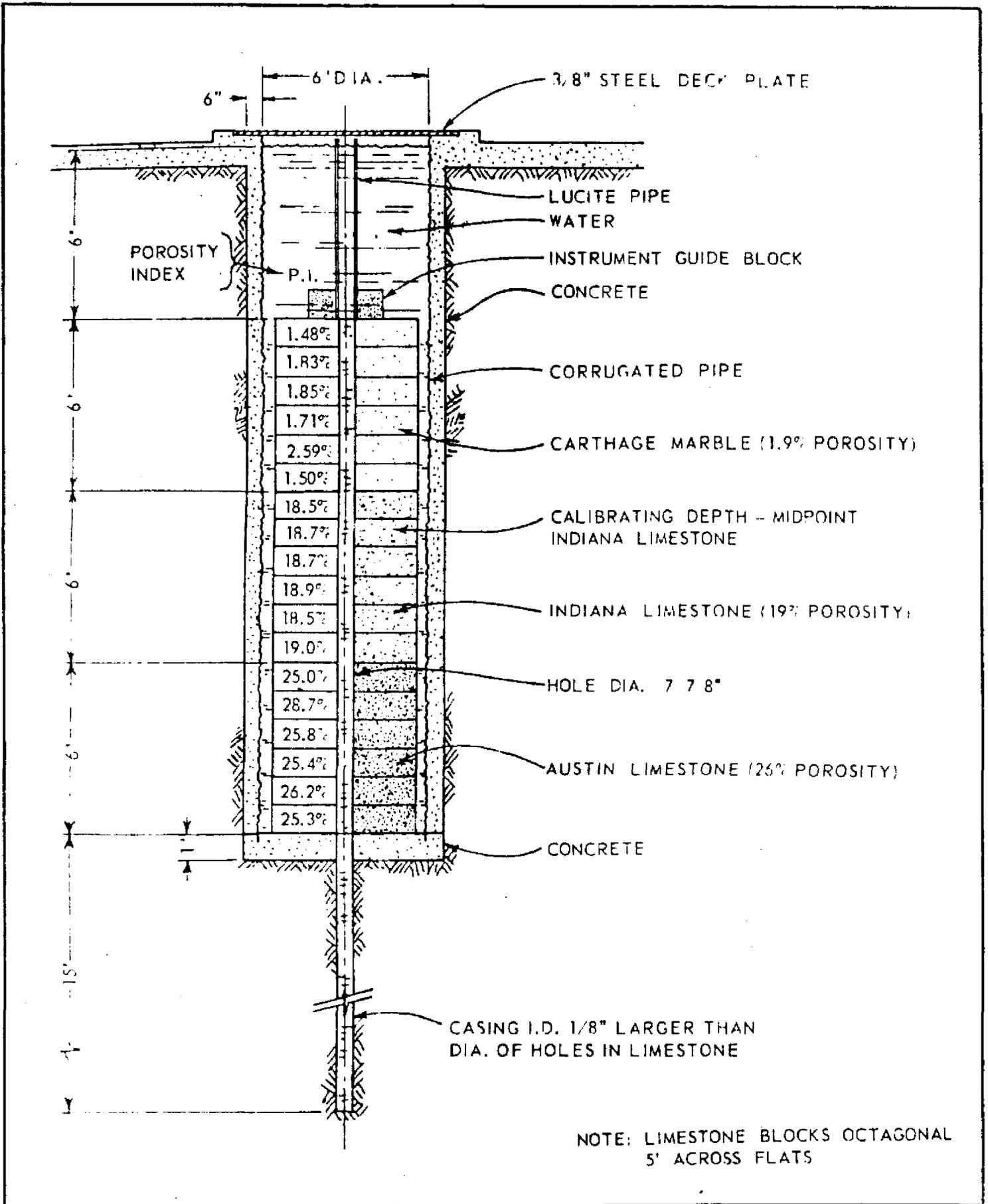
Figure 7 - Neutron Log Calibration Pit (taken from API, 1971)
