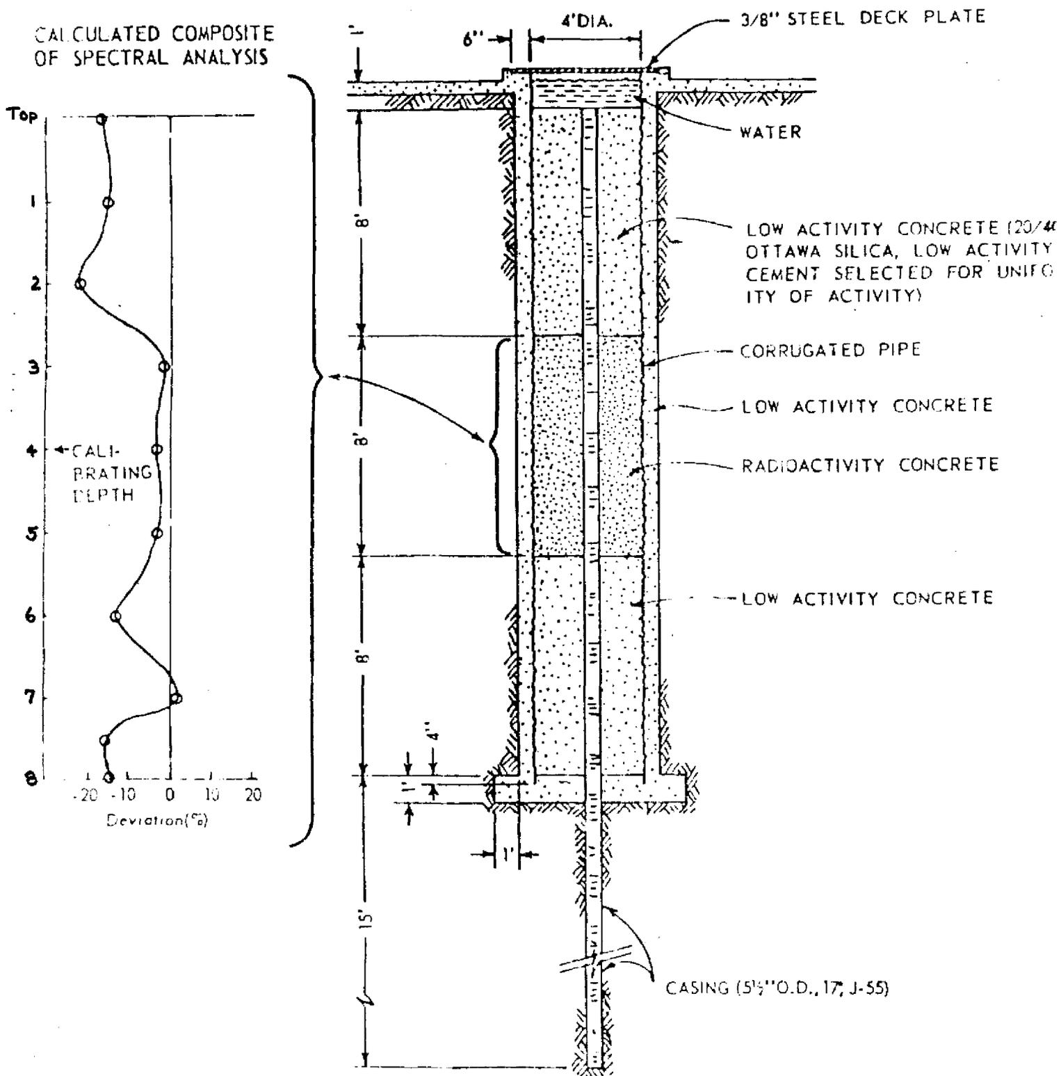
Figure 6 - Gamma Ray Calibration Pit (taken from API, 1971)
