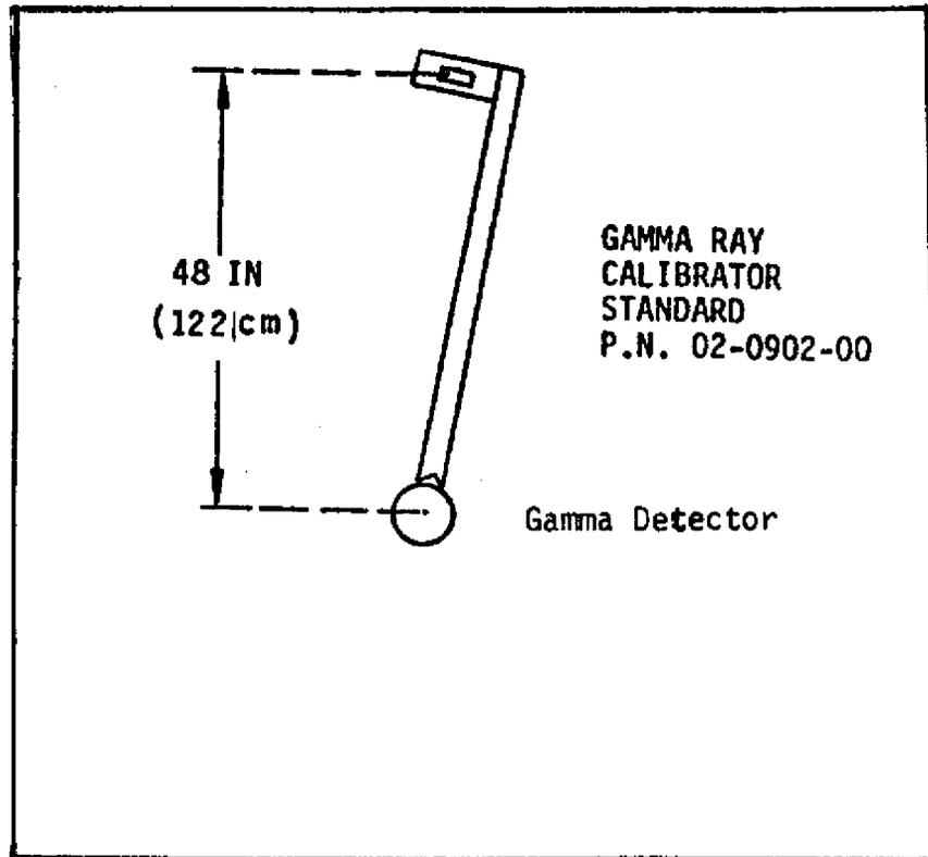
Figure 3 - Setup for the Gamma Ray Calibrator (taken from G.O.I., 1978).
