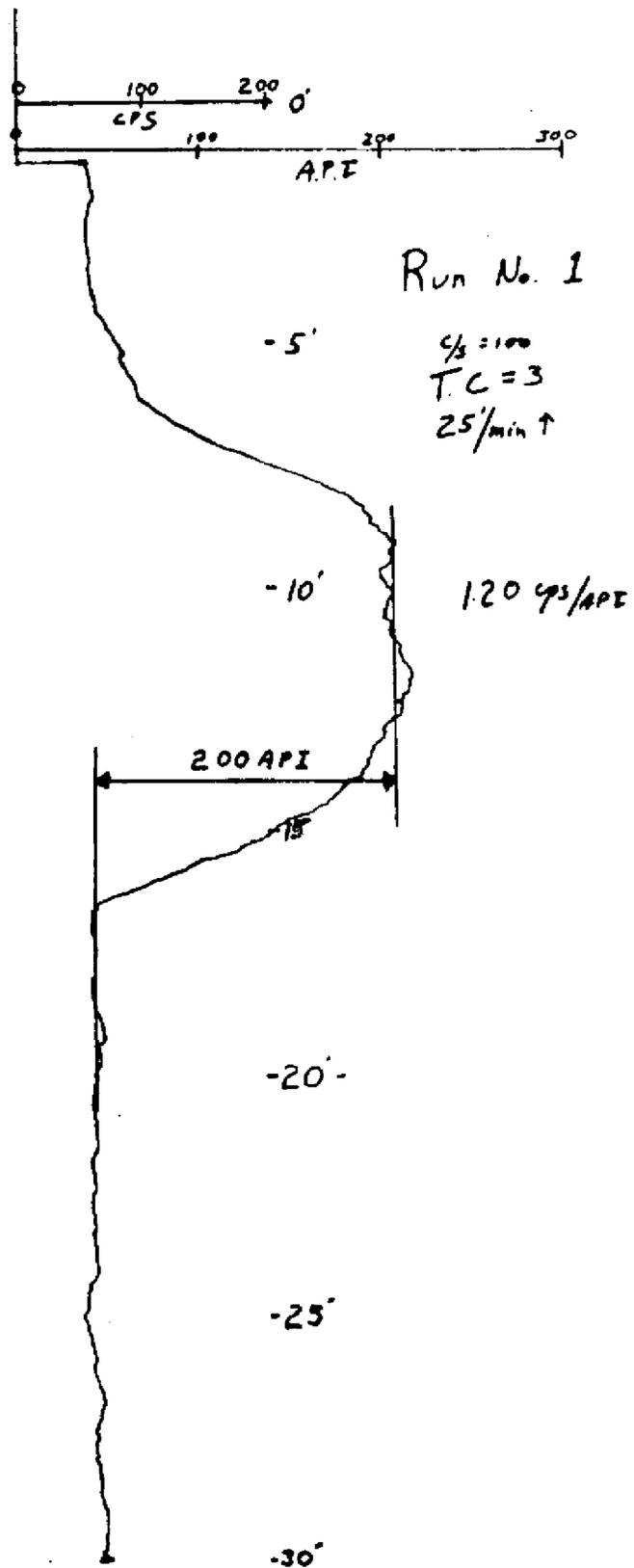
Figure 8 - Natural gamma ray Run #1 in the gamma ray API Test Pit, University of Houston.
